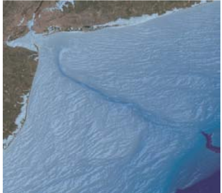
Image 2.1. An example of a bathymetric surface in the New York Bight, showing the change in depth with distance from shore and the complexity of the seafloor across the shelf. The Hudson Shelf Valley is prominently visible in the center of the model as the area of darker blue extending from New York harbor (top left) towards the shelf edge (bottom right). Coastal managers and engineers use bathymetric surfaces to assess shipping lanes, identify fish habitats, lay undersea cables and find sand and gravel resources. The bathymetric surface shown here is the the NOAA Coastal Relief Model (CRM), draped over a derived hillshade layer to highlight bathymetric variation. Terrestrial imagery is the ArcGIS Online World User Imagery layer (ESRI Online).
