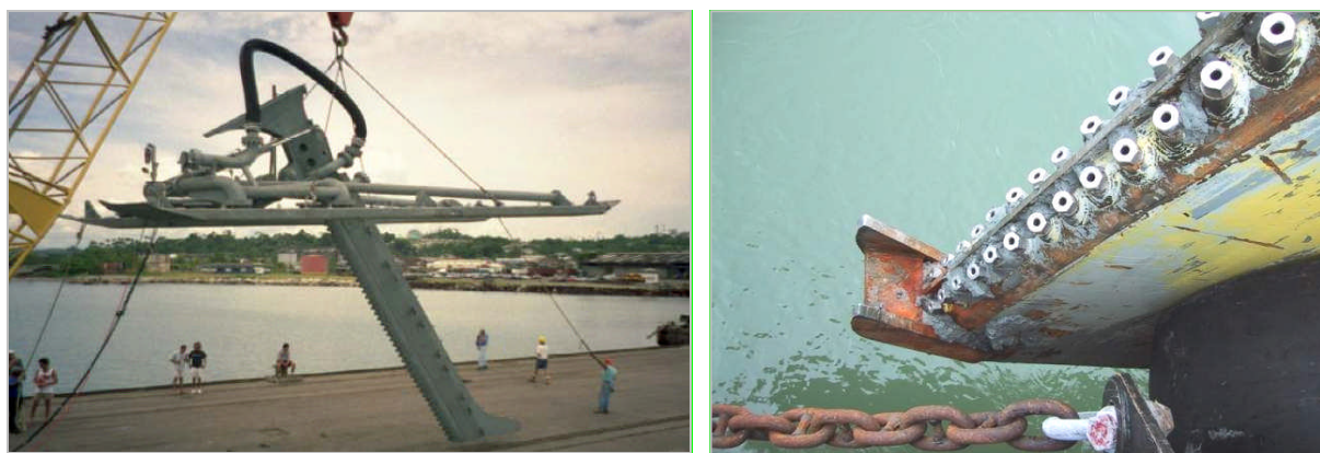
Fig. 12 Left: Jetting plough with 5 m blade extended (LAWRENCE 2002), right: close view of jetting plough blade (MOLL 2006)
