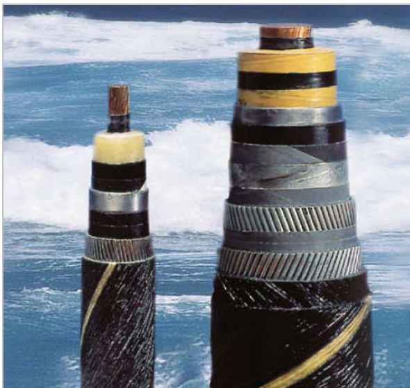
Fig. 7 Submarine power cables manufactured by ABB; left: polymeric HVDC Light cable for DC and paper-insulated mass-impregnated cable for HVDC, right: XLPE-insulated three-core and single core-cable for AC (ABB 2006b).
