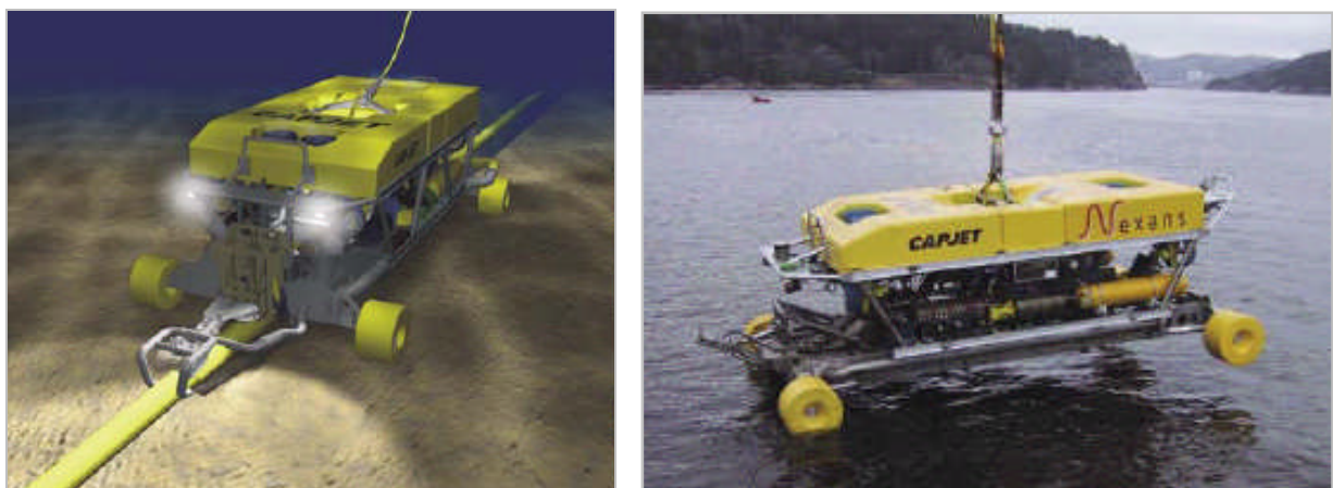
Fig. 10 Nexans' Capjet system trenches cables and umbilicals by fluidising the seabed materials. The vehicle docks on the cable or pipeline, follows these objects and can start and stop trenching operations at any point along the route. Simultaneous back-fill with the fluidised materials is achieved during the trenching operation. It can be employed in shallow waters as well in water depths up to 2000 m (NEXANS 2005).
