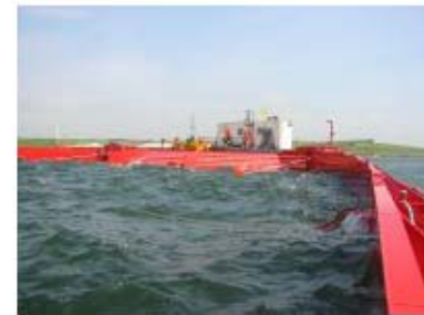
FIGURE 6 Wave Dragon Overtopping Device (Source: Wave Dragon 2005)
