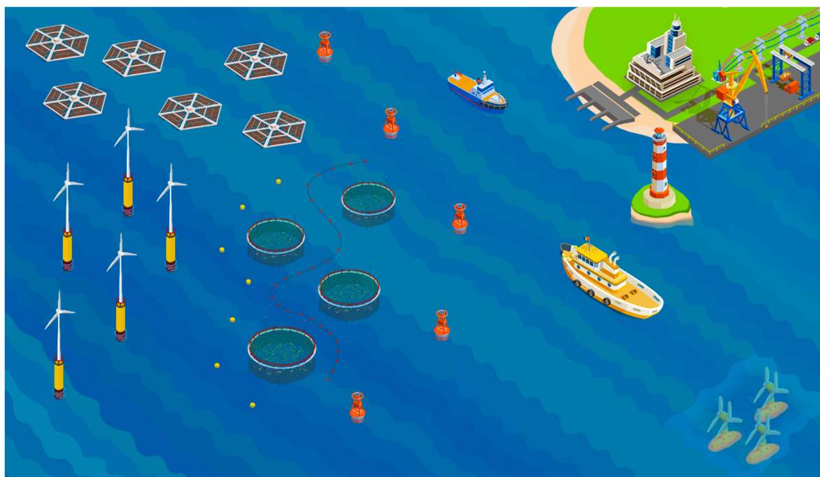
Figure 1. Graphic representation of all studied elements that can coexist in a MUP: aquaculture, offshore wind energy, offshore solar energy, marine energy represented by a tidal energy converter (for the elaboration of this image, the vectors were taken from [13]).
