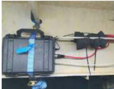
Figure 6. Detail of the airborne sound acquisition system installed inside the WAVEGEM device.
