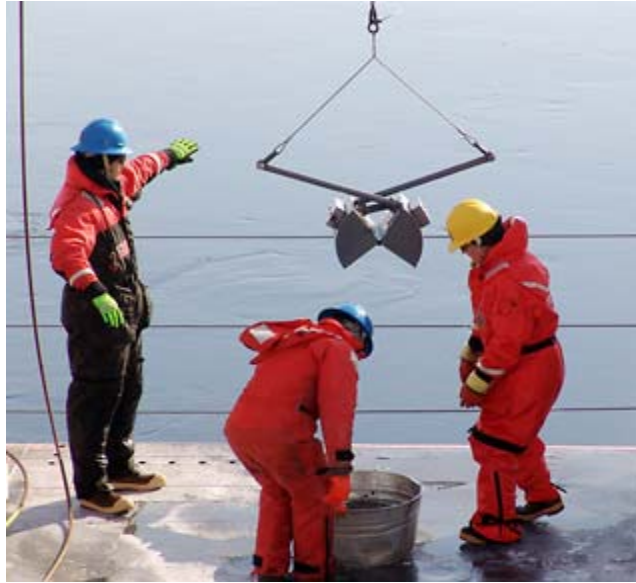
Figure 2: Van Veen grab used to take seabed samples
