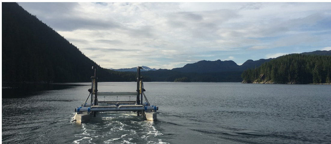
Mavi Innovations Mi1 floating turbine deployed at Blind Channel, British Columbia.
