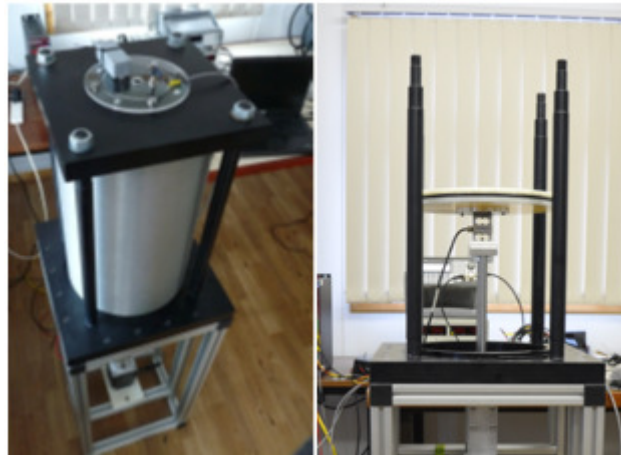
Figure 14: picture of the pneumatic orifice calibration test rig in UCC-HMRC (closed on the left and open on the right)
