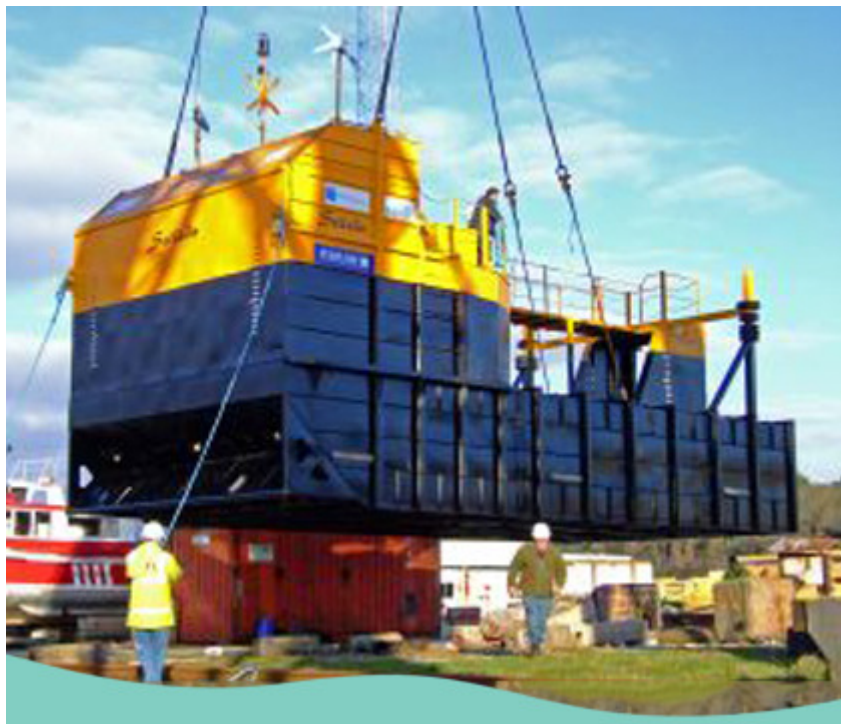
Figure 1: Picture of the OEbuoy quarter scale model tested in Galway bay test site.
