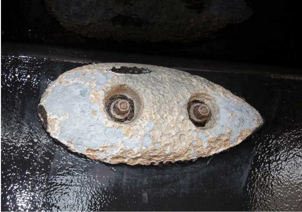
Figure 9: example of a corroded zinc anode on a ship hull (setsail.com)
