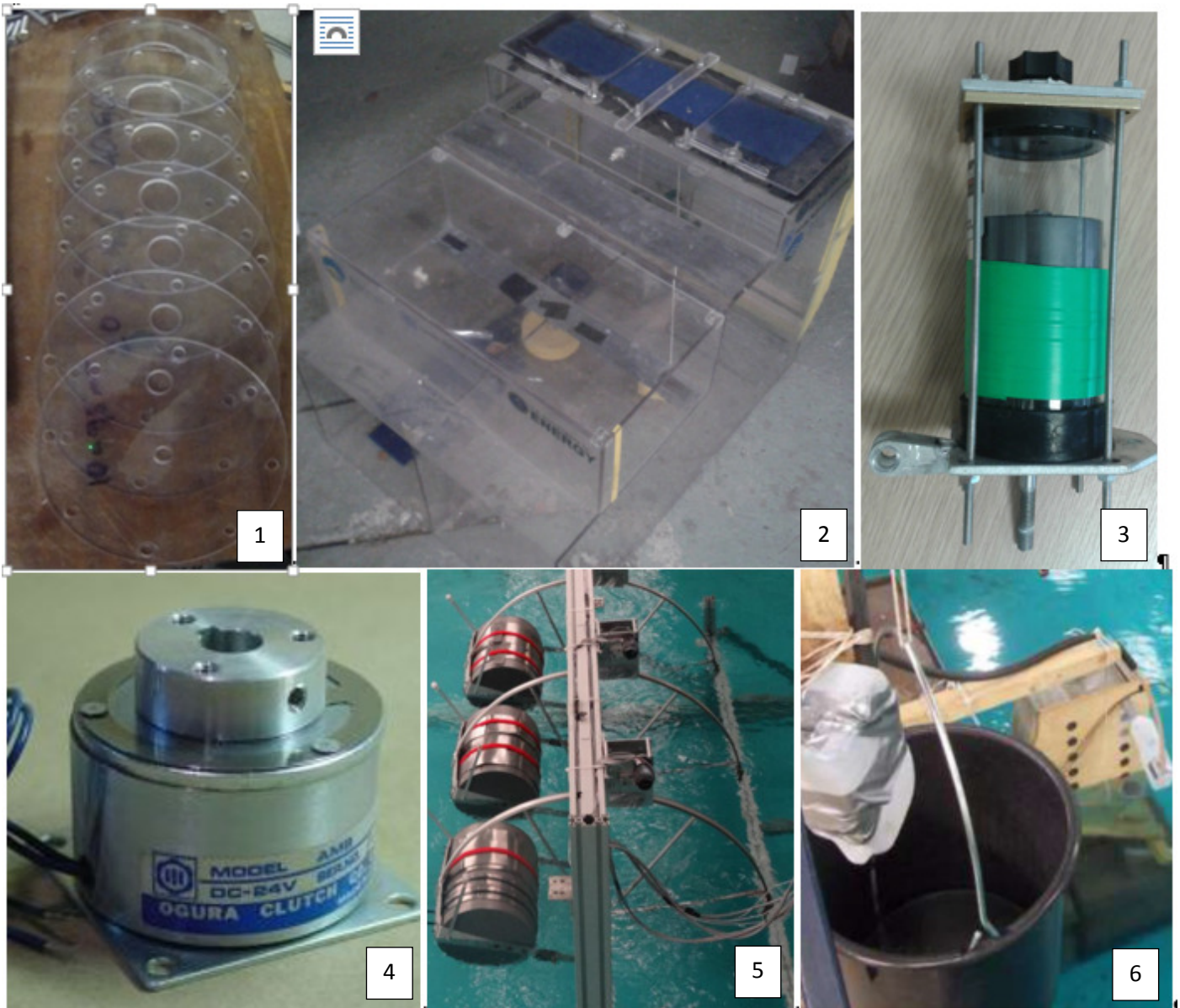
Figure 7: PTO system at stage 1-2 from left to right: pneumatic orifices (UCC) porous membrane (UCC), pneumatic piston damper (UCC), electromagnetic break (OGURA website), Elevated tank (UCC, MARINET “Wavepump” trials), servomotors (UCC, MARINET “W2P” trials)
