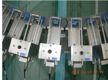
Figure 50 Top view of some AMOEBA's absorber elements
