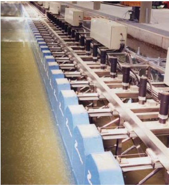
Figure 9 'Classical' piston-type wave maker (Equimar)
