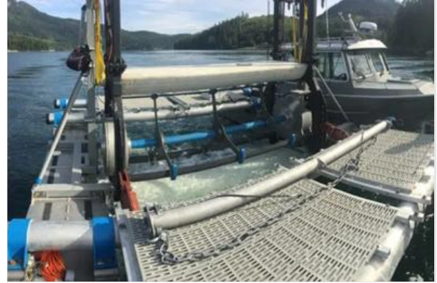
Mavi Innovations crossflow turbine
