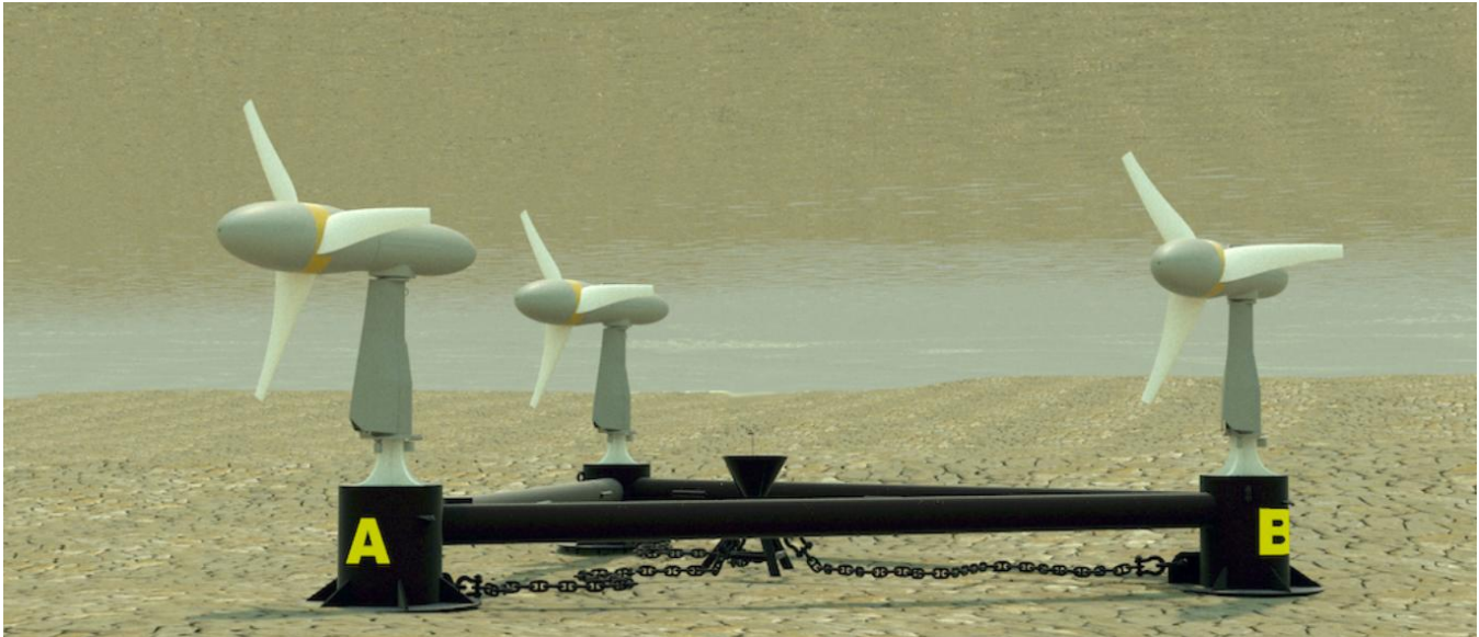
Figure 16: Verdant Power Turbines on a Triframe Base
