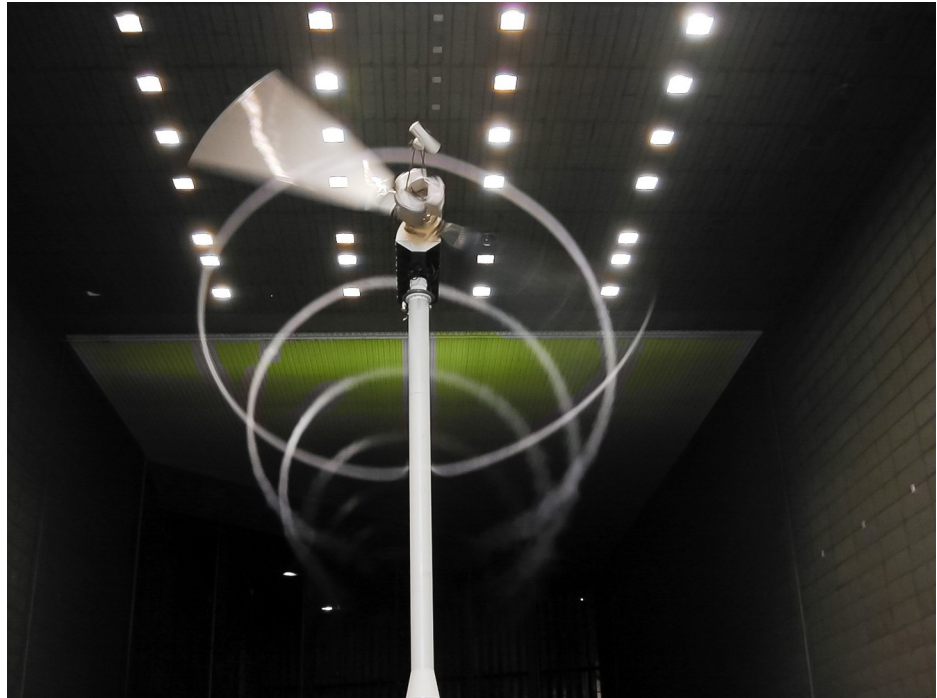
Fig 2. Smoke visualization of a blade-tip vortex at the national aeronautics and space administration's ames research center 40-by-80-ft wind tunnel. The visible helical vortex indicates the region of low pressure caused by the blade-tip vortex. Note that this visualization was performed under low-turbulence conditions in a wind tunnel, allowing the vortex to advect downwind with the mean flow with its helical structure intact. In the atmosphere, where the turbulence intensity is typically much higher, the vortex structure is commonly unrecognizable within one rotor diameter downstream of the rotor plane. Photo by Lee Jay Fingersh, National Renewable Energy Laboratory, 55062.
