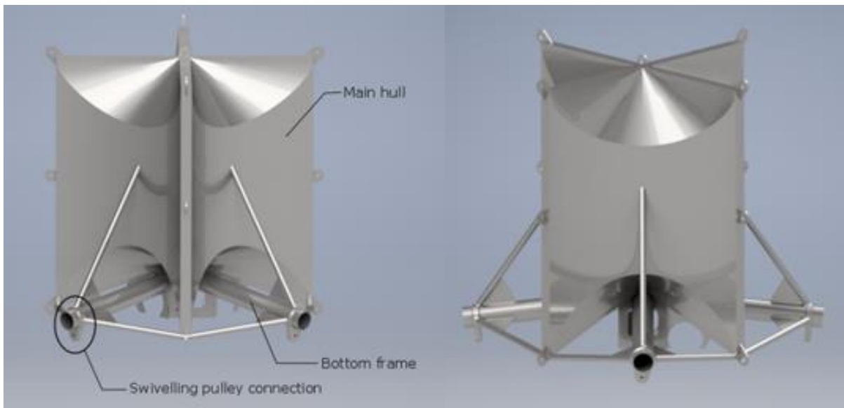
Figure 7: Front and side view of the Laminaria WEC (drawing)
