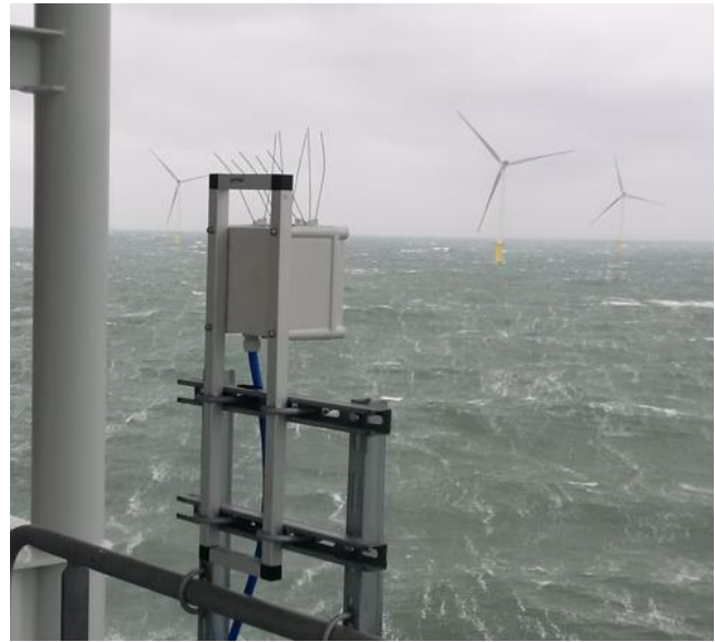
Figure 2-3. Ultrasound microphone at Gemini Buitengaats OHVS.
