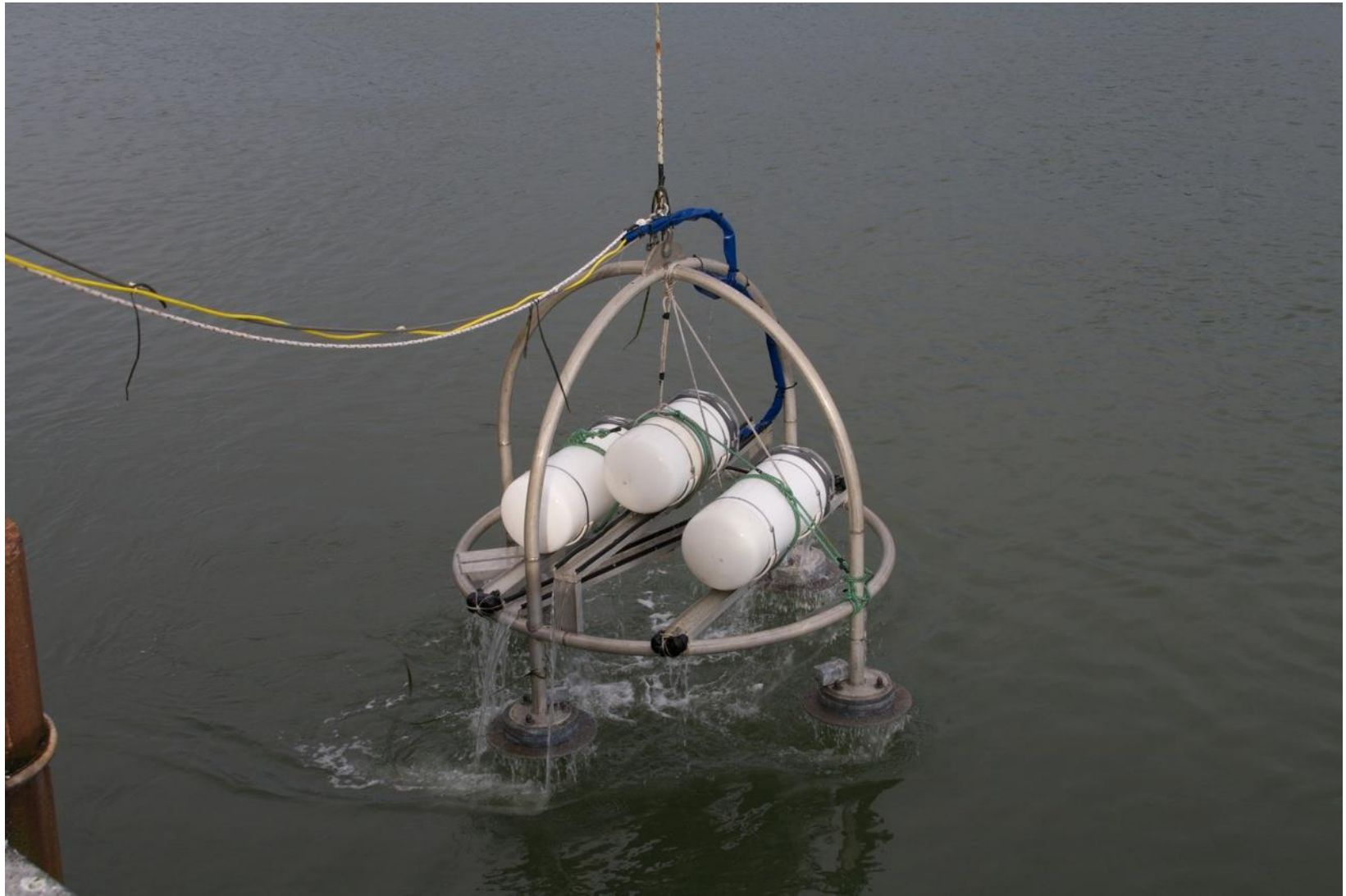
Figure 4: Waterproof housings containing Airmar signal generator and batteries mounted on Lander anchor.
