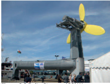
Figure 6.3 Delta Stream; 400kW Demonstrator ready for deployment at Ramsey Sound and subsequent monitoring.
