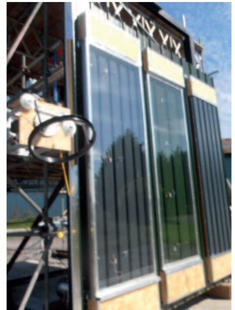
Figure 2.7 Three selected collector units tested at SBEC.
