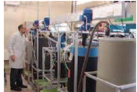
Fig 4.10 Advances made by SERC have resulted in up to 37% increase in biomethane yield through the integration and optimization of a biohydrogen reactor.
