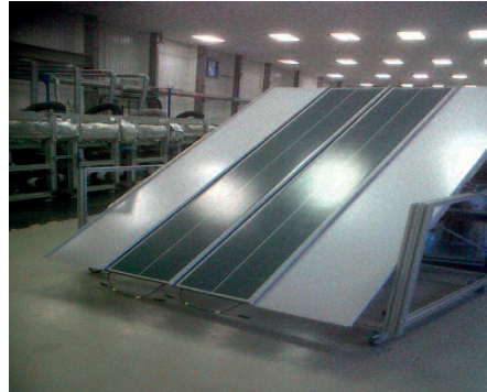
Figure 2.3 Thin film PV cells are encapsulated and bonded to a metal cladding system.
