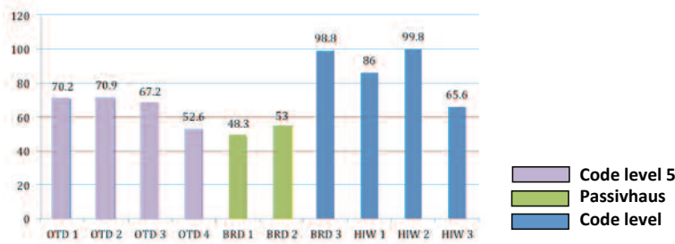
Figure 2.46 A cross site comparison of total annual energy consumption delivered energy (kWh/m2/annum).
