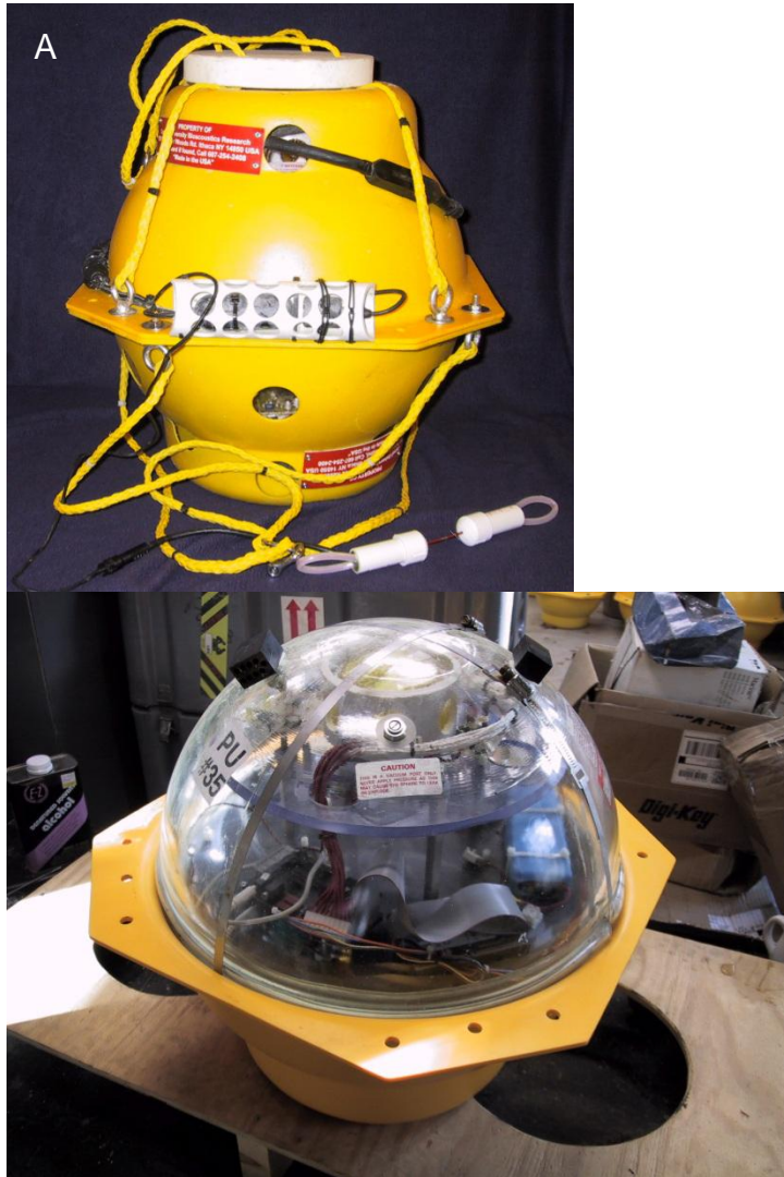
Figure 1. (A) External and (B) internal views of the Marine Autonomous Recording Unit (MARU) used for sound data recordings in this project.
