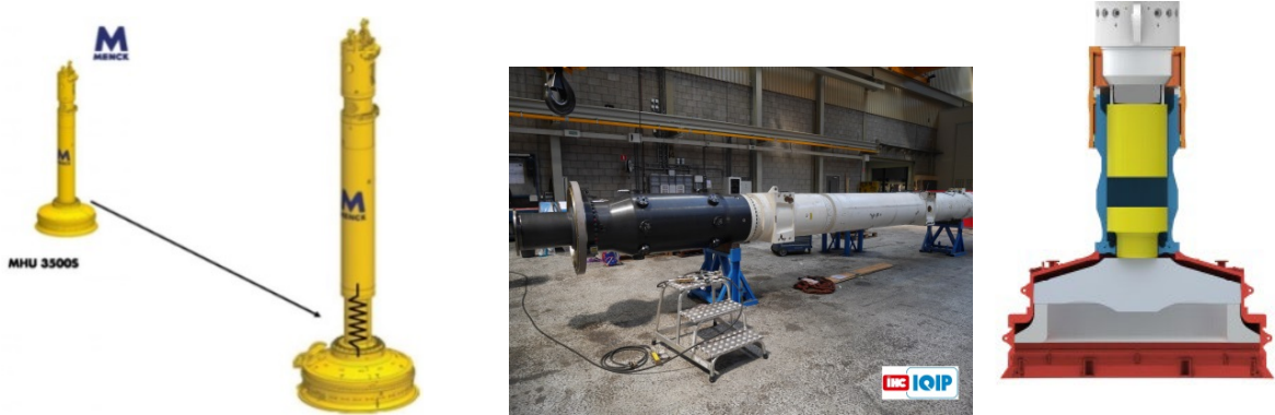
Fig. 8. View of a standard hydraulic impact hammer and a modified hammer (right) with a MENCK Noise Reduction Unit (MNRU) added between ram weight and anvil (left, © MENCK) and IHC S-90 hammer with added PULSE system in black housing (middle) and cross-sectional view (right, © IHC IQIP).
