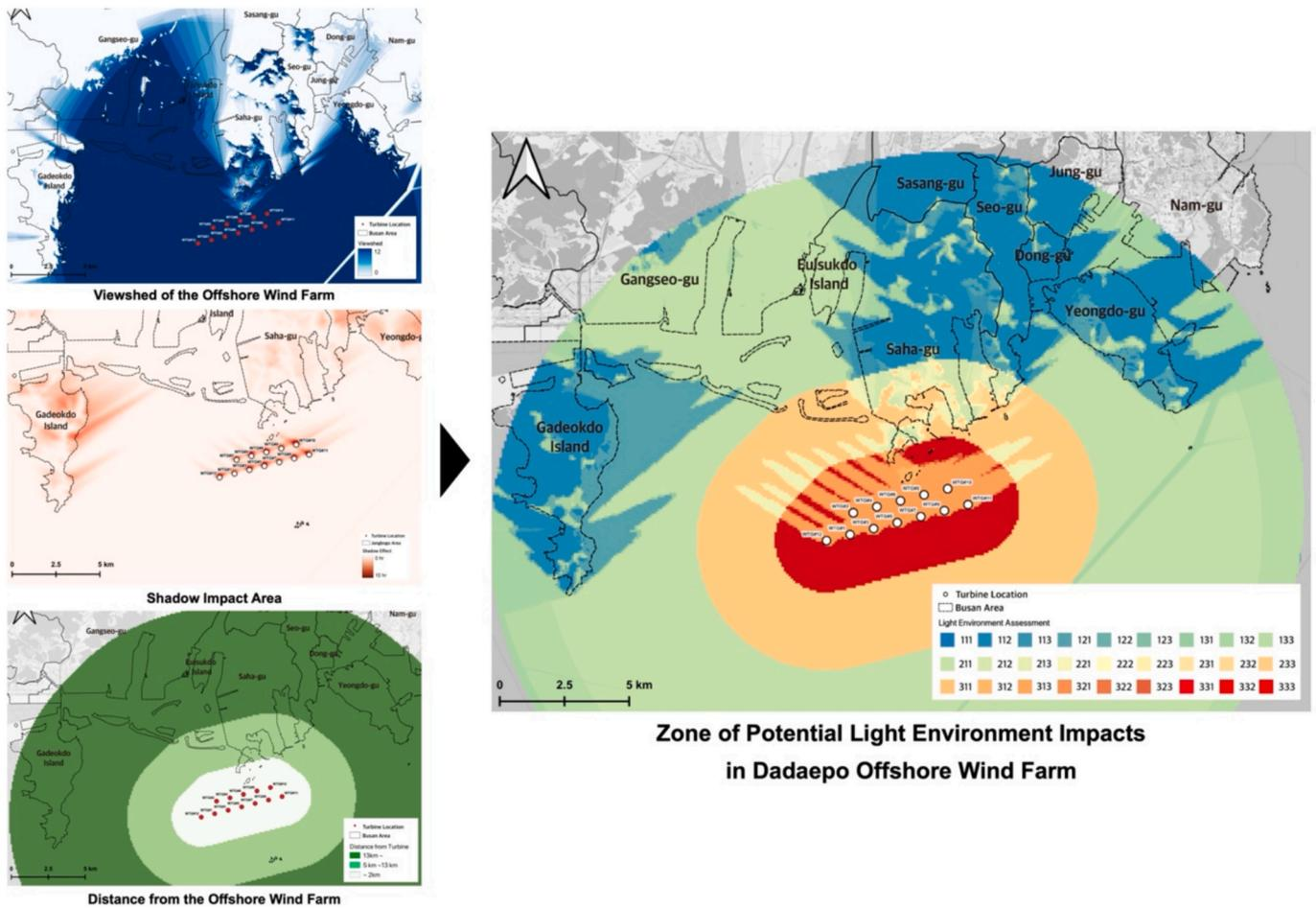
Fig. 5. Potential light environment impact zone in Dadaepo offshore wind farm.
