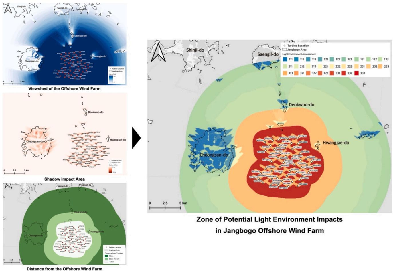
Fig. 4. Potential light environment impact zone in Jangbogo offshore wind farm.
