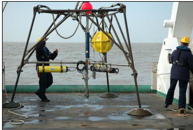
Figure 9. PoD vertically mounted on a tripod (image: J.Backers, MUMM).
