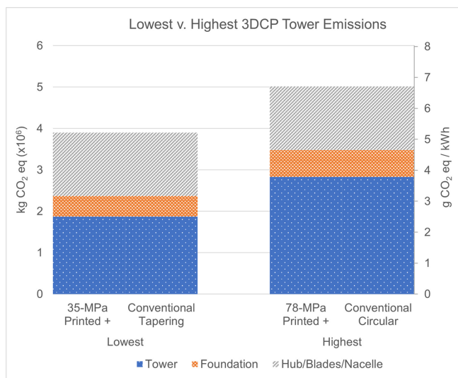
FIGURE 11 | Lowest and highest tower and foundation combinations with respect to global warming potential (GWP) and grams of CO 2 equivalent per kilowatt-hour (kWh). This estimate does not include shared features for the tower and foundation subassemblies.
