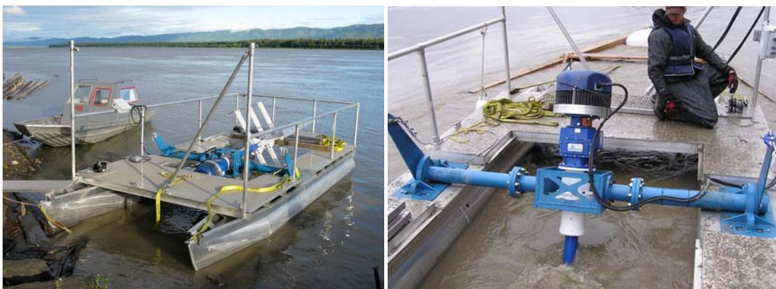
Figure 6. New Energy EnCurrent Turbine (on left) and deployed in the Yukon River (pictures courtesy of New Energy Corporation and Tom Ravens)
