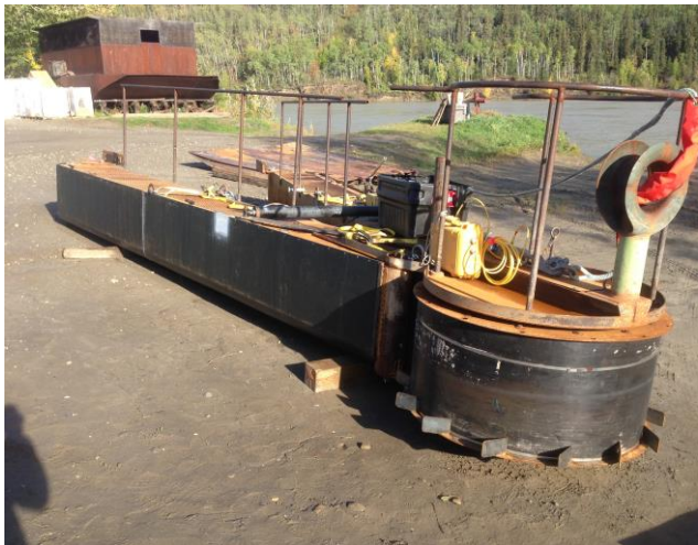
Figure 1. The RDDP debris sweep (front cylinder) and pontoons with plastic sheet covering to reduce contact friction between the RDDP and debris.
