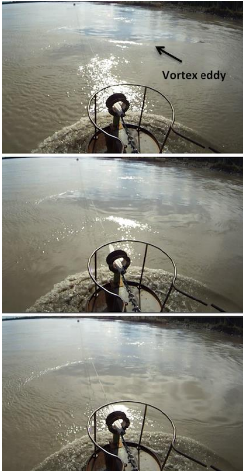
Figure 23a. Vortex eddy (~ 3 m) moving downstream toward the RDDP on the Tanana River.
