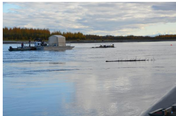
Figure 8. AHERC test barge, with the Oceana hydrokinetic turbine on deck, moored behind the RDDP as a debris object floats by.
