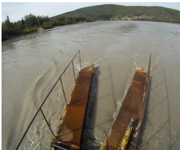
Figure 23b. Downstream view of RDDP-generated turbulence.
