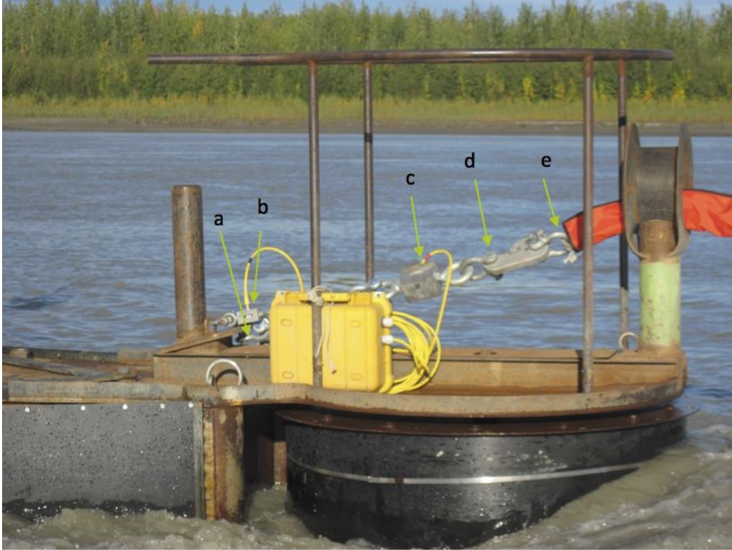
Figure 4. Load cell connection setup: (a) shackle connection to RDDP; (b) high-resolution load cell (2,000 lbf/9 kN); (c) high-capacity load cell (20,000 lbf/90 kN); (d) quick release mechanism; (e) connection to mooring tether line.
