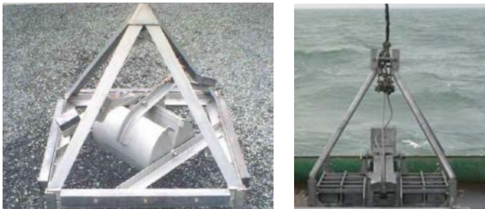
Figure 5-7. Example of a day grab (left) and hammon grab (right). Taken from Guerra & Freitas, 2012.
