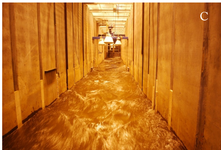
Figure 2-5 a-c. Test flume with turbine in (panels a and b) and out (panel c). Visible in panel a are the turbine, lights, PIT antennas, cameras, and hydrophones (see schematic, Figure 2-1 and 2-2). Note that the turbine created some head differential, which affected flow velocities in those zones (Table 2-1, Figure 2-6.)
