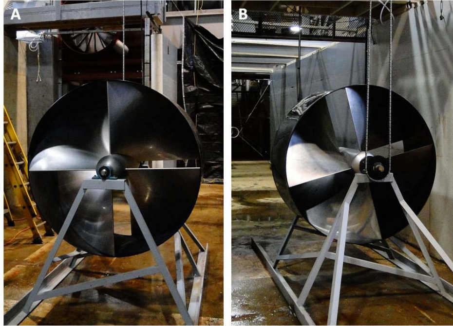
Figure 2-4 Downstream (A) and upstream (B) views of the Welka UPG turbine installed in Alden's large flume test facility
