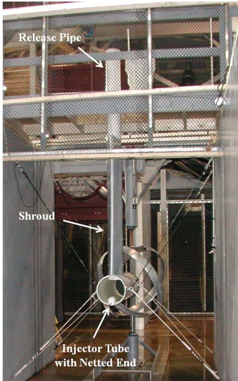
Figure 2-7 Downstream view of the test fish release system configured for survival testing with the Lucid turbine
