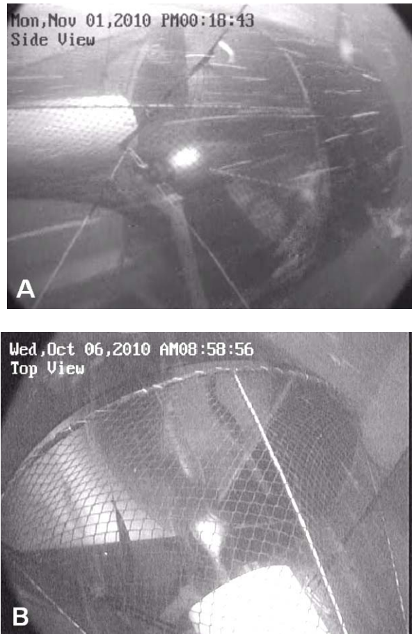
Figure 3-6 Side camera view (A) showing a fish being struck by a blade and top view (B) showing fish swimming immediately upstream of the blade sweep during testing at an approach velocity of 1.5 m/s.
