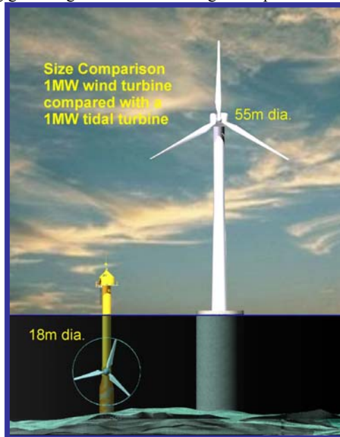
Figure2: Size comparison of a 1MW wind and tidal turbine ((c) Marine Current Turbines Ltd.)
