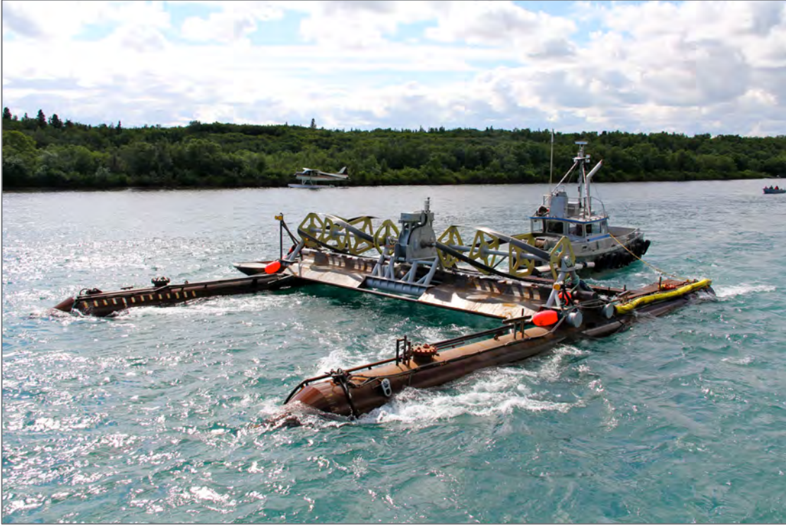
Figure 2.1. Photograph of the ORPC RivGen® device.
