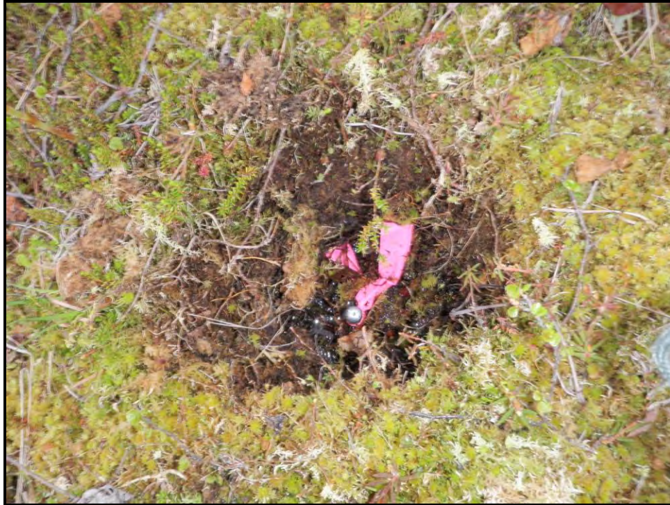
Figure 13 – Monument HK-4. \frac{1}{2} inch x 8 foot steel rod with bullet top.
