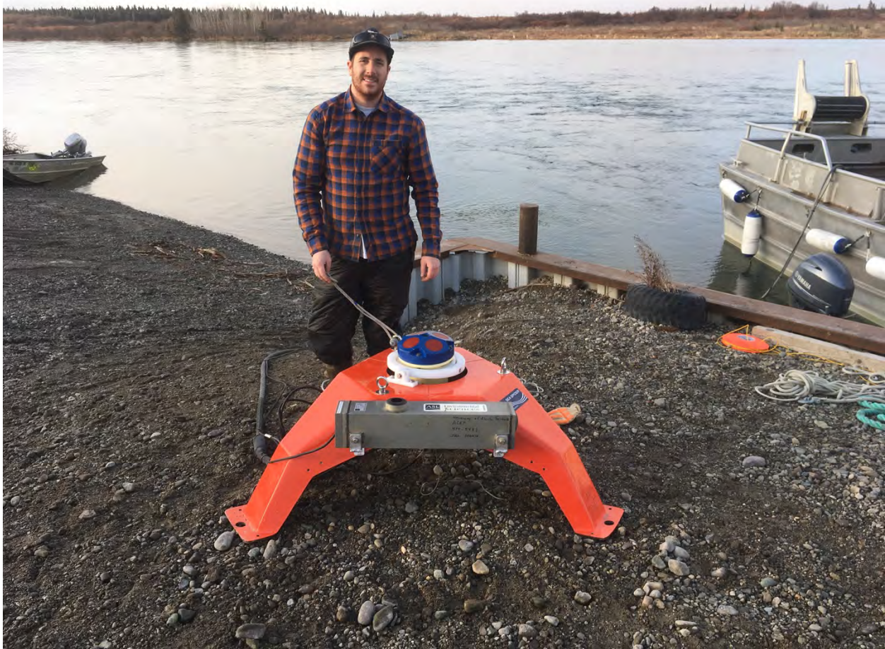
Figure 3 . UAF personnel with the ADCP and SWIP mounted on an orange fiberglass “Sea Spider” frame. The instruments ready for loading on the F/V EG in Igiugig in November, 2016.
