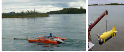
Figure 2: Doppcat platform for down looking Nortek Aquadopp velocity profiler (left) and sounding weight platform for Nortek Vector velocimeter (right) at Igiugig, AK.
