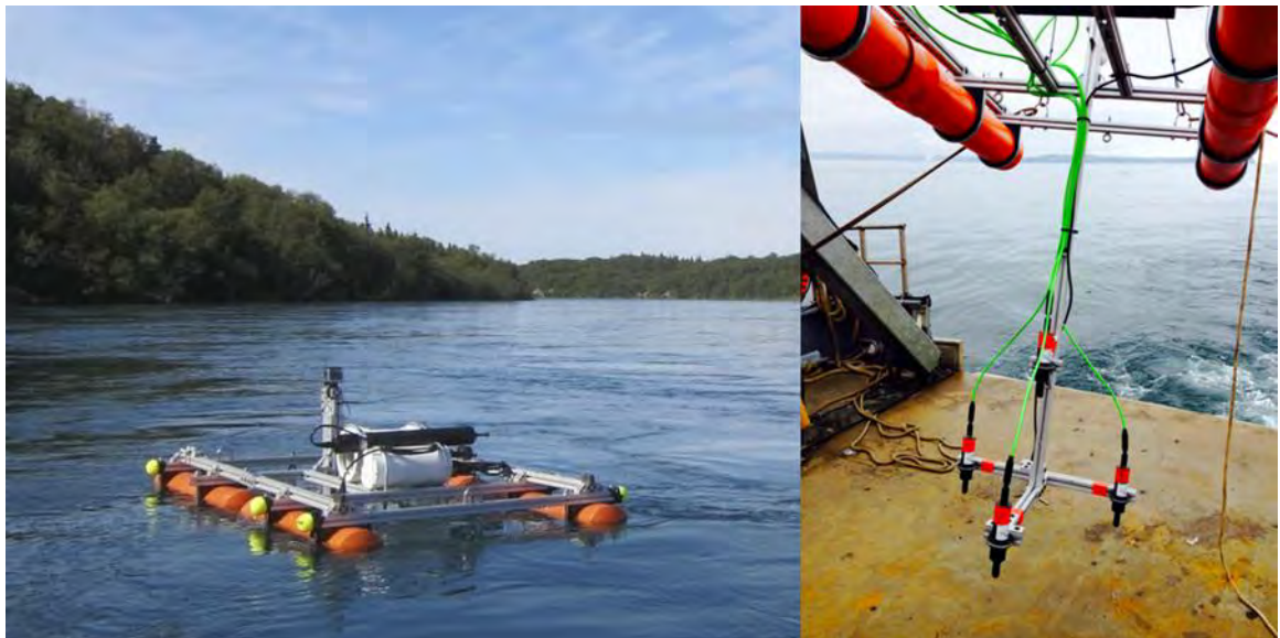
Figure 5: The RivRaft during deployment on the Kviachak, chandelier submerged (left). The chandelier with hydrophones and Doppler velocimeter in lowered position (right).
