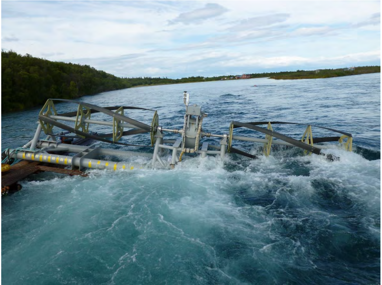
Figure 3: Deployment of the RivGen ® 1.0 device on the Kvichak River in 2014
