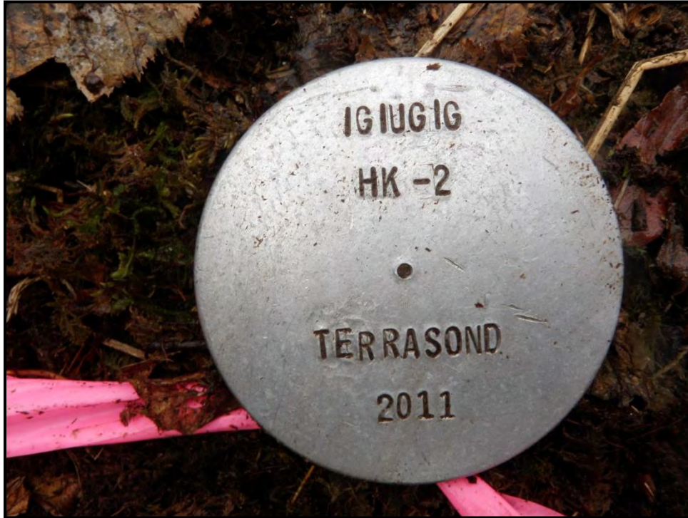
Figure 9 – Monument HK-2. 3 ¼ inch aluminum cap on rebar. (Destroyed.)
