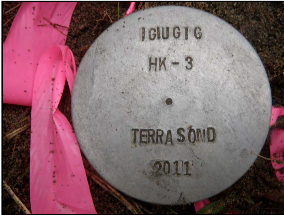
Figure 11 – Monument HK-3. 3 ¼ inch aluminum cap on rebar.
