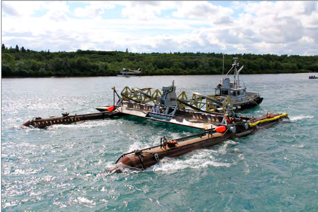
Figure 2.1. Photograph of the ORPC RivGen® device.
