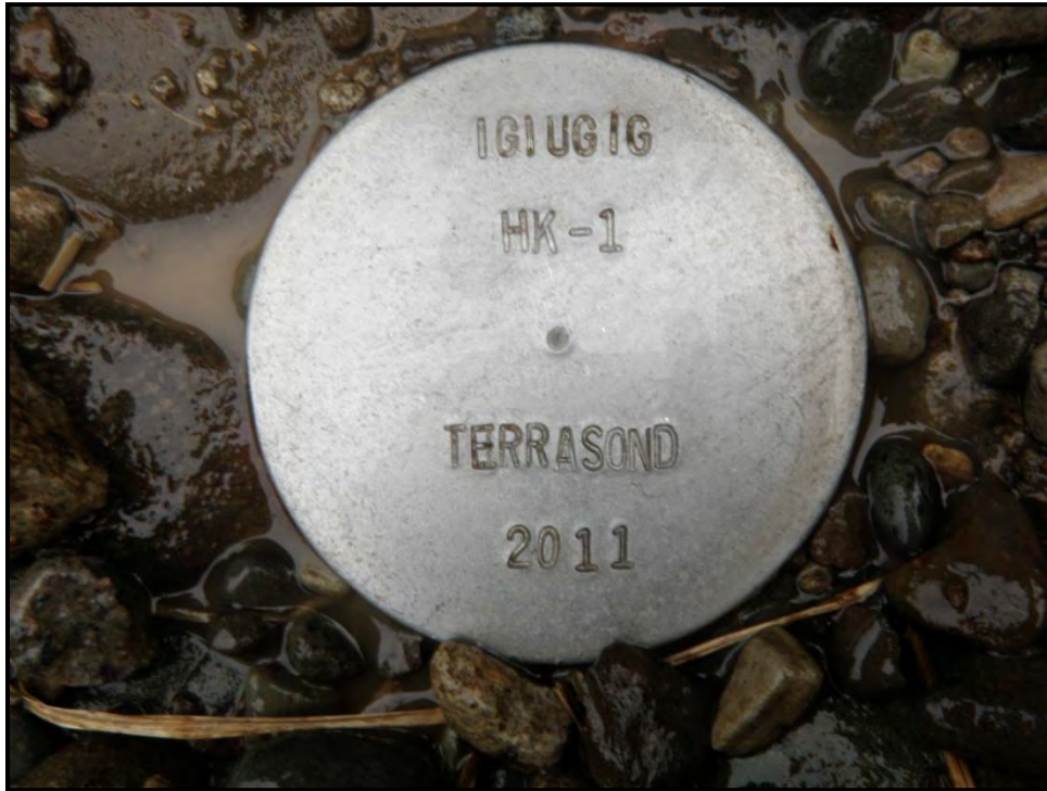
Figure 5 – Monument HK-1. 3 ¼ inch aluminum cap on rebar.
