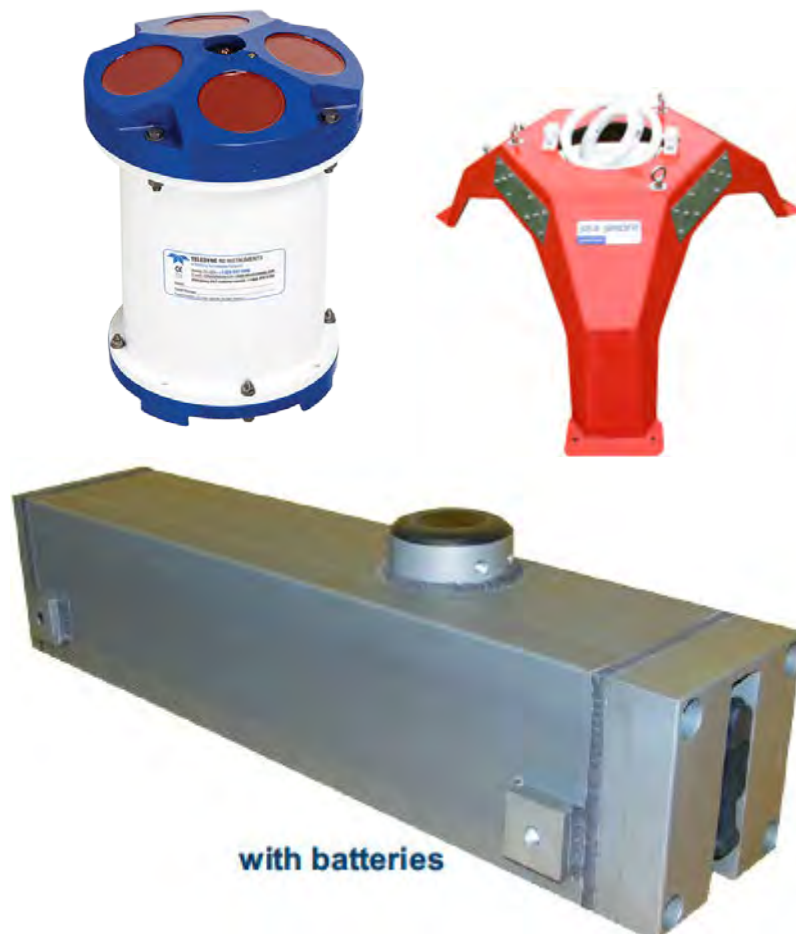
Figure 20. Top Left: a TRDI Workhorse Sentinel ADCP. Image courtesy of TRDI, Inc. Top Right: An Ocean Science "sea spider" mooring frame. Bottom: An ASL Environmental Sciences SWIP with extended battery case. The Sea Spider frame will be equipped with 150 lbs of lead weights (50 lbs on each tripod leg) to keep the package moored to the river bed.
