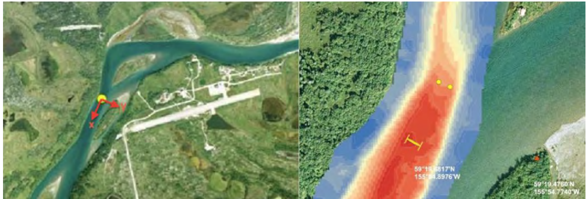
Figure 3: RivGen Site. The village of Igiugig on the Kviachak River, flowing from Lake Iliamna (left, out of frame). The turbine location and coordinate system are shown with satellite view of the village of Igiugig (left). Local bathymetry and locations of upstream anchors can be seen (right). Position of turbine is approximate.
