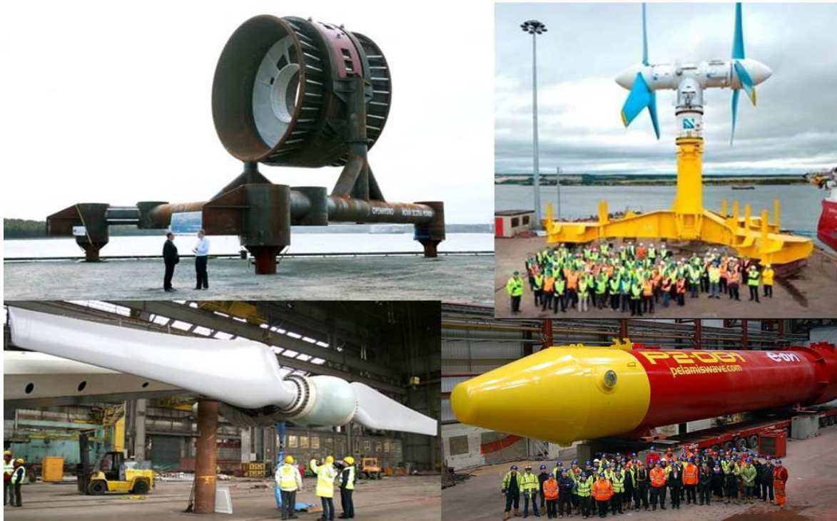
Figure 1. Examples of three leading tidal-stream turbines and one wave device. People in the pictures provide scale. Top left: OpenHydro ( www.openhydro.com ), top right: Atlantis AK-1000 ( www.atlantisresourcescorporation.com ), bottom left: MCT SeaGen ( www.seageneration.co.uk ), bottom right: Pelamis Wave Power ( www.pelamiswave.com ).
