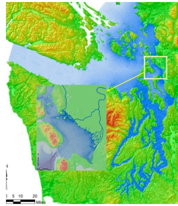
Figure 2. Example of grid for application of FVCOM in a tidal estuary, allowing for detailed simulation of energy removal from tidal energy devices (Puget Sound, WA USA)
