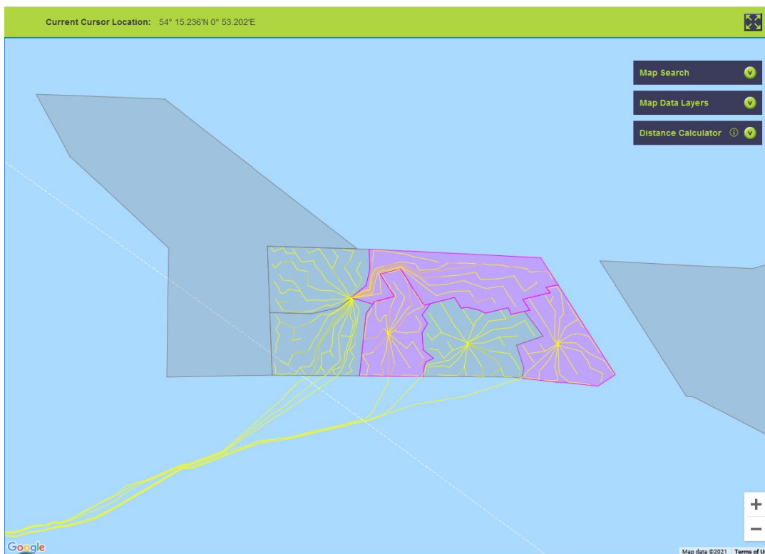
Figure 1.2. An example of inter-array and export cables from a European large-scale offshore windfarm. The cable network shown here is from the ‘Hornsea One’ (165 turbines, 1386 MW) and ‘Hornsea Two’ (174 turbines, 1218 MW) offshore windfarms in the southern North Sea off the east coast of England, UK. Image sourced from kis-orca.org and turbine information from 4coffshore.com (accessed February 2021).
