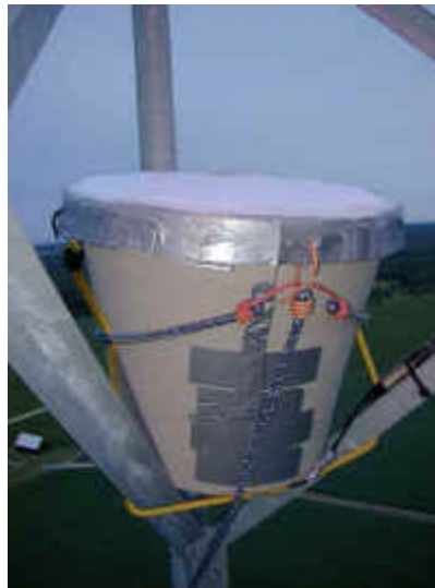
Figure 8. Microphone mounted near the top of 67-meter high meteorological tower. Note farmhouse in lower left.
