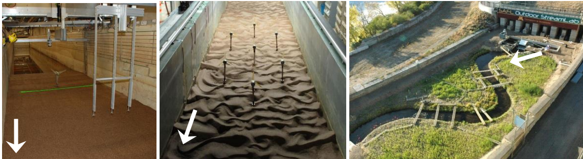
Figure 1: (Left): The SAFL Main Channel showing 0.5m diameter turbine. (Center): SAFL Tilting Bed Flume with 7 turbine staggered array during small-scale turbine experiments. (Right): Photograph of the SAFL Outdoor StreamLab (OSL) meandering stream.
