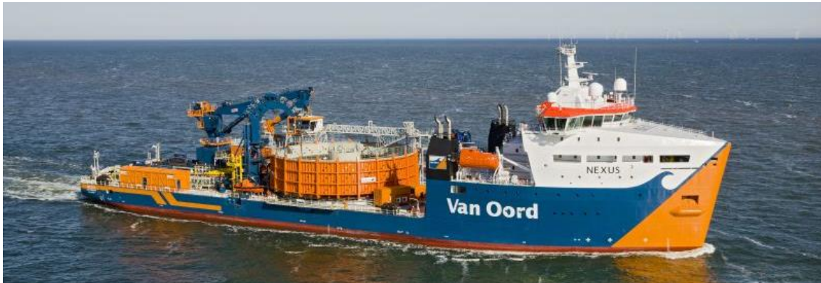
Figure 4.8 Example of a cable-laying vessel. Source: Van Oord
