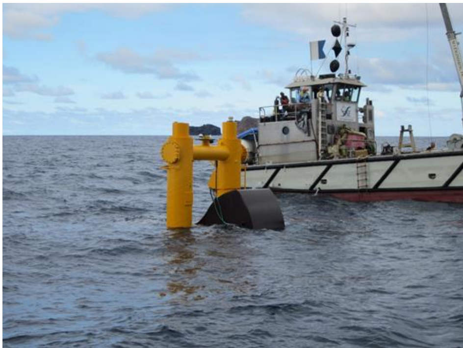
Figure 1.8. Northwest Energy Innovations (NWEI) Azura WEC, during deployment in late May 2015 at the Wave Energy Test Site (WETS) 30m test berth. Sea Engineering's vessel Huki Pau is seen, just after deployment.
