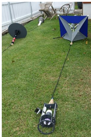
Figure 4.3. University of Washington SWIFT drifting hydrophone system, shown with a heave plate configuration on the left and with a drogue on the right.
