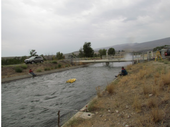
FIGURE 4. SNL STAFF CONDUCTED CROSS-SECTION VELOCITY MEASUREMENT USING AN ADCP AT THE DOWNSTREAM OF THE IES TURBINE
