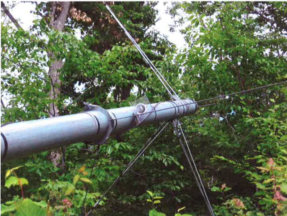
Figure 3. Example of Bat-Hat mounted on met tower, while tower is lowered.
