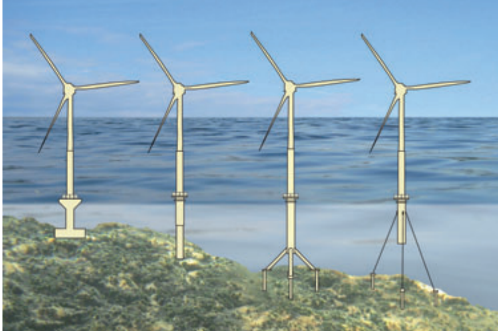
Figure 4: Offshore foundation options – the figure demonstrates the four main types of offshore wind power foundations. From left to right: Gravity, Monopile, Tripod, Floating. © C. Wilhelmsson.
