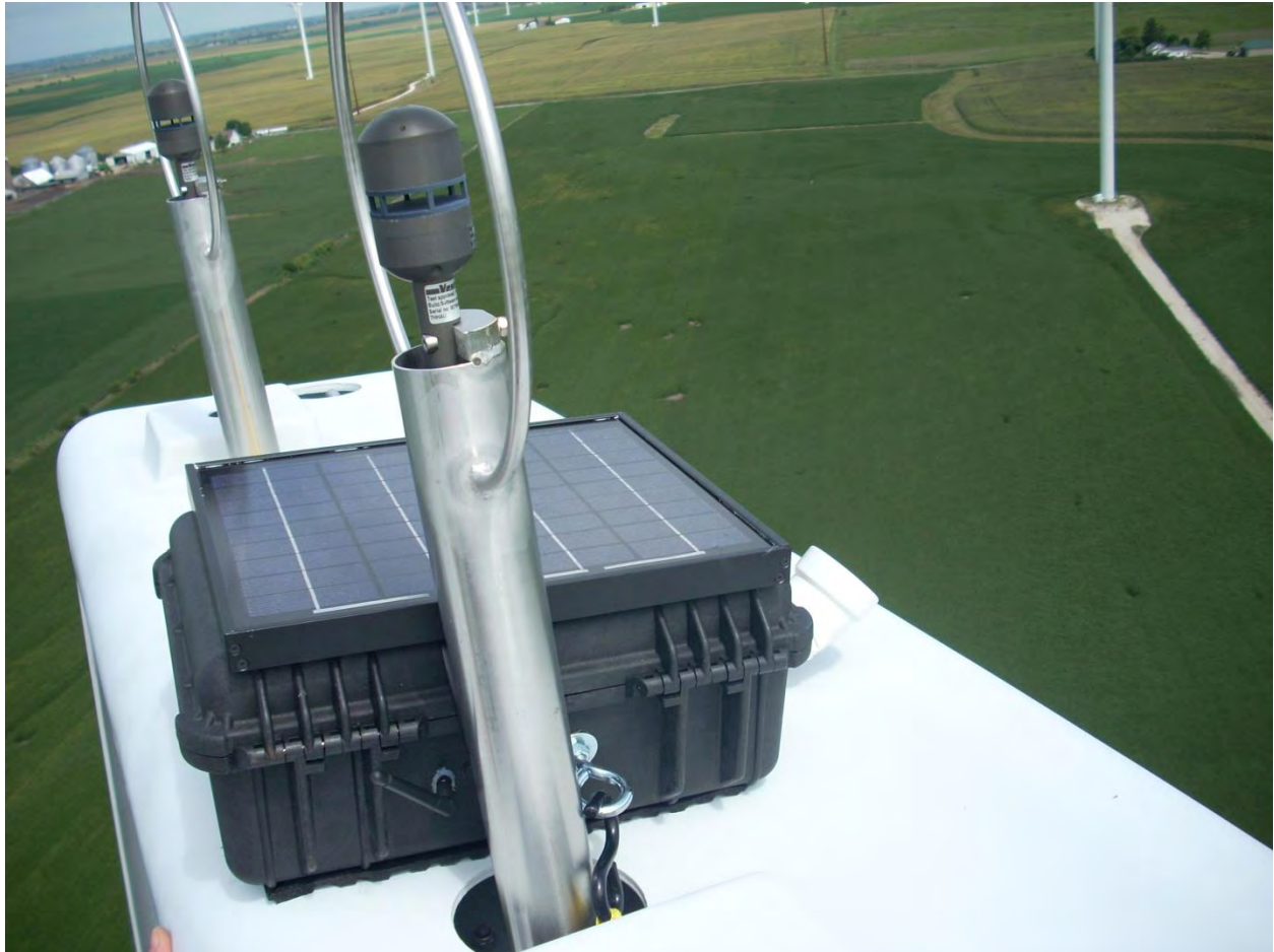
Figure 8. Anabat unit mounted on the nacelle of a wind turbine at the Fowler Ridge Wind Farm.
