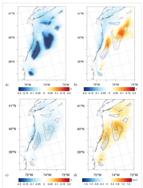
Figure 4. Same as figure 2, but for: (a) temperature above hub height ( $\sim$ 200 m AMSL), (b) temperature below hub height ( $\sim$ 90 m AMSL), (c) temperature at the surface, and (d) sensible heat fluxes at the surface (note that a positive change in downward negative heat flux means a reduction in its magnitude).
