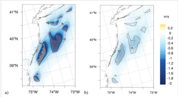
**Figure 2.** Wind speed changes due to the wind farms (WF–NF) in Domain 2, averaged over 3 summer months: (a) at hub height ( $\sim$ 120 m AMSL) and (b) at the surface. The red-dashed line shows the contour of 0.5 m s<sup>-1</sup> wind speed deficit, which is considered as the edge of the wake.
