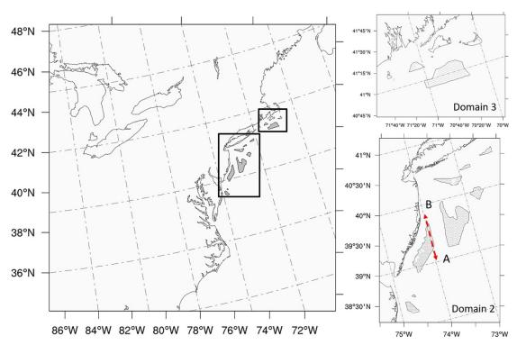
**Figure 1.** Computational domains: parent domain with  $400 \times 400$  grid cells (4 km resolution), Domain 2 with  $260 \times 170$ , and Domain 3 with  $105 \times 132$  (1.33 km resolution for both). The turbine locations are shown with grey dots and the edges of the planned WEAs with grey lines. Results for Domain 3 are presented in the supplementary appendix.
