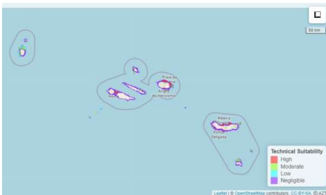
Figure 9. Spatial distribution in Azores of suitability levels, based on technical factors, for developing wave energy projects.
