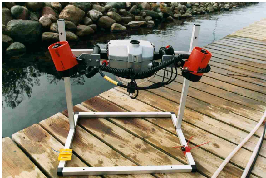
Figure 2.4 Equipment used for digital photography of the fouling community at Nysted Offshore Wind farm in September-October 2003
