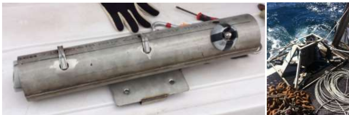
Figure 73. Scour monitor in bracketing (left); Seabed frame and AWAC (right).
