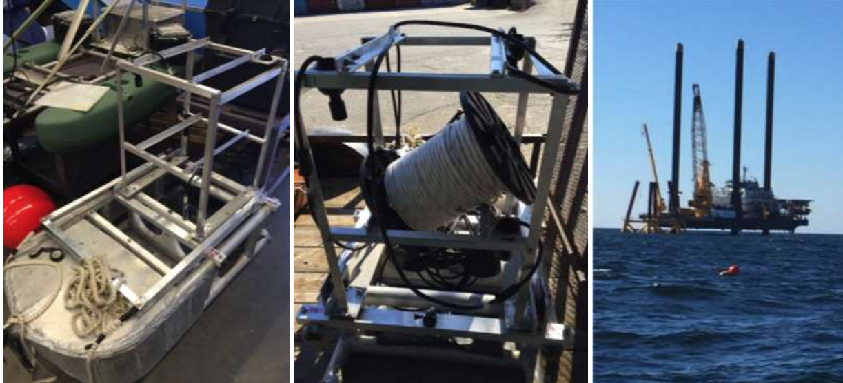
Figure 41. Images of the geophysical sled before deployment (left and center). These two photographs show the tetrahedral array of hydrophones with a spacing of 0.5 m (1.6 ft). Photo of the surface floats for the sled with WTG 4 in the background (right).
