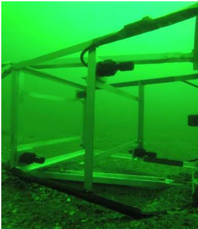
Figure 42. An underwater photo captured via a GoPro camera mounted on the bow of the sled shows the tetrahedral array of hydrophones is maintained despite the sled landing on its side.
