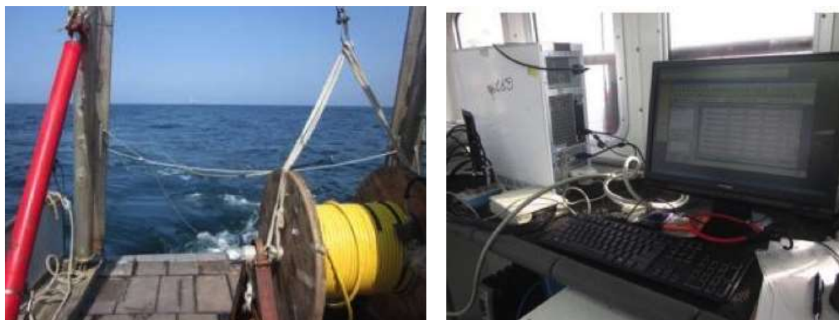
Figure 34. Towed array spool configuration (left) and data collection station installed in the vessel lab (right).
