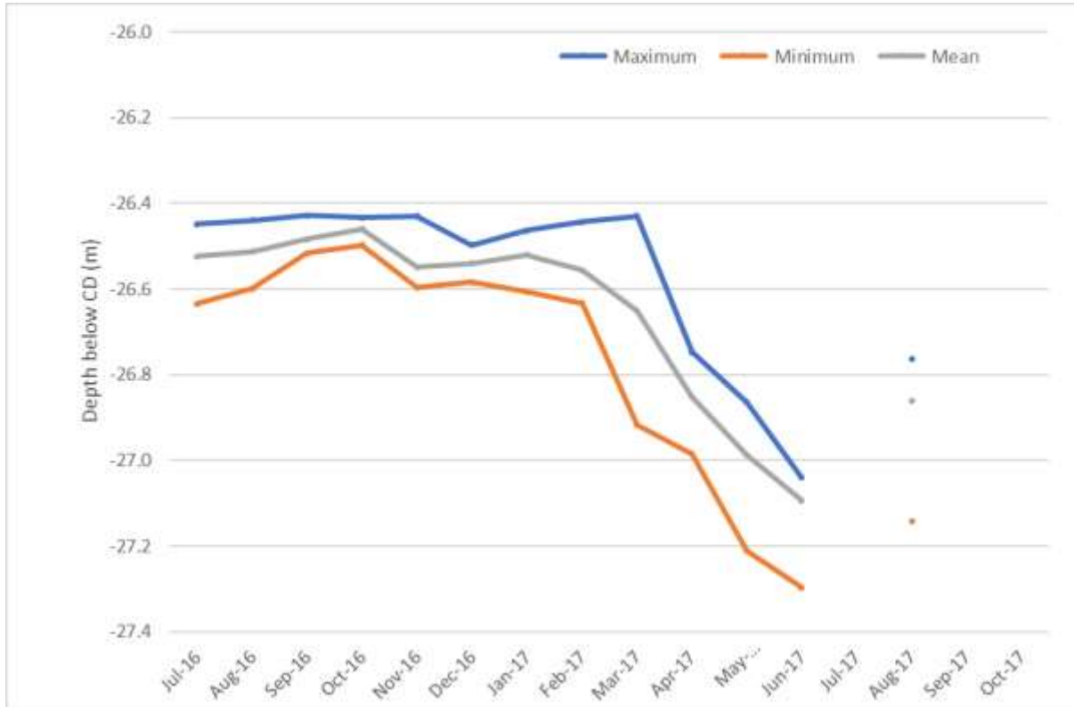
Figure 81. SE Beam 1 scour depth.
