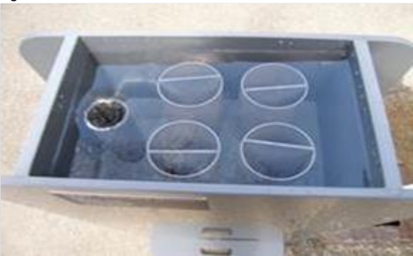
Figure 5: DNV GL / KEMA monitor- PVC riser tubes and fouling plates
