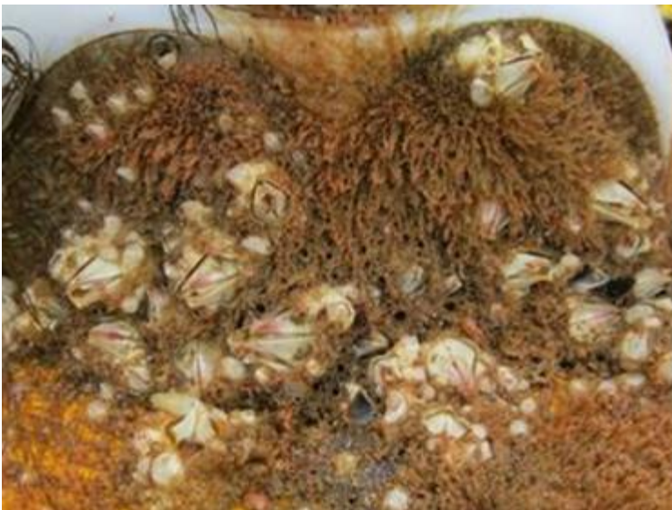
Figure 1: Image showing macrofouling on an ADCP after 8 months in Orkney
