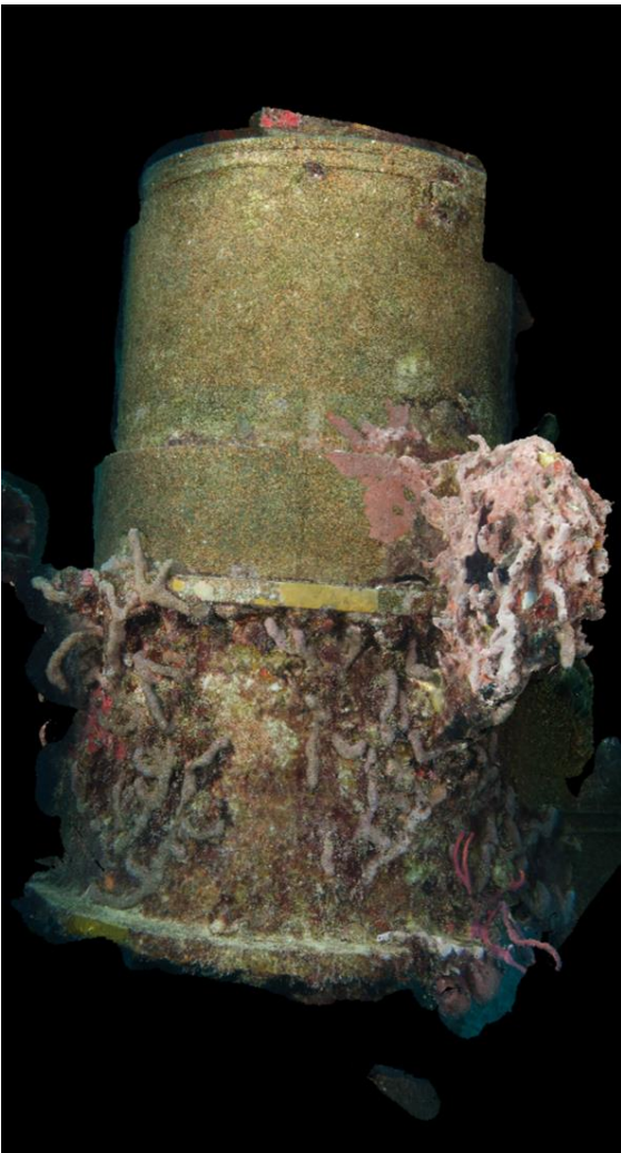
Figure 2: A reconstruction of a biofouled underwater structure using Multiview photogrammetry techniques © Andrew Mogg, The Scottish Association for Marine Science & National Facility for Scientific Diving.
