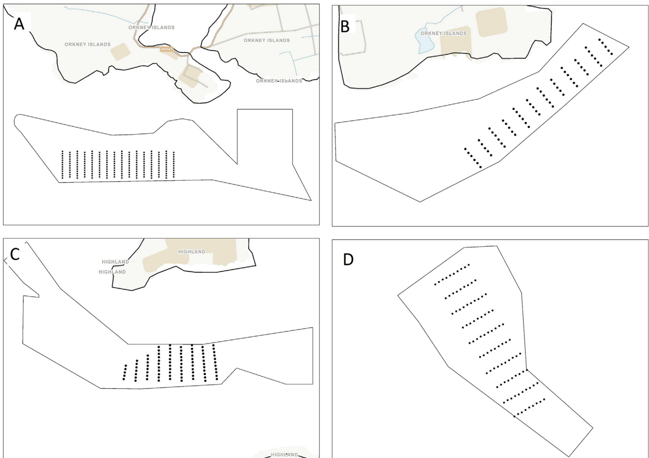
Fig. 10. Tidal energy turbine array layouts for (A) the Brims tidal array, (B) the Brough Ness tidal array, (C) the Meygen array and (D) the Ness of Duncansby array. Turbines are marked as black dots and the licensed areas as black lines.
