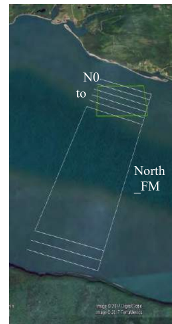
Figure 4: Contemporary survey grid. The green square represents the CLA. White lines show one complete grid, with transects at the CLA (N0-N5) and reference (S1-S3) sites connected by cross-channel transects (South_CW and North_FM).
