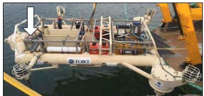
Fig. 1 FAST-1 sensor platform developed by FORCE and deployed at the FORCE test site. White arrow indicates location of AZFP transducer. Photo credit: Tyler Boucher.
