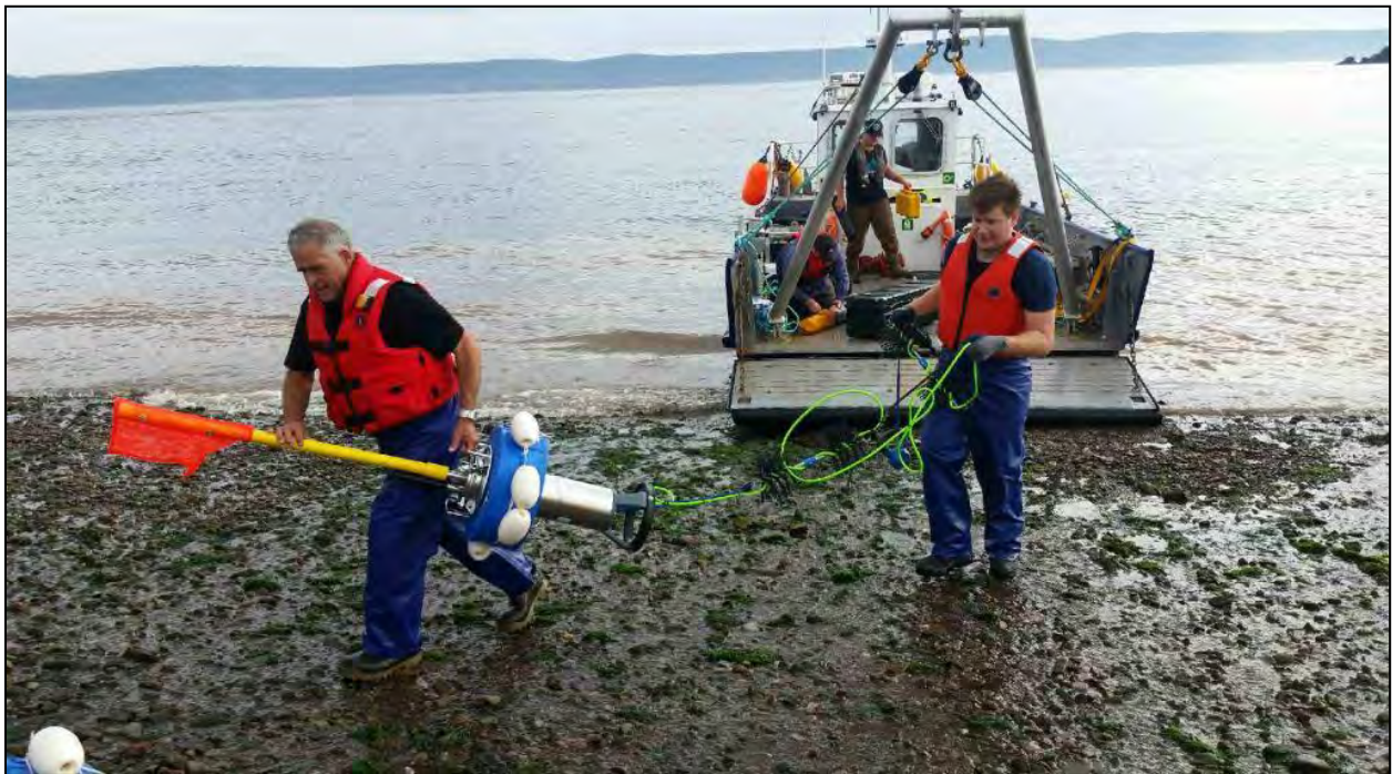
Figure 8: Tyler Boucher, FORCE ocean technologist, and crew of the Tidal Runner demobilize after completing data collection using drifting hydrophones in support of the marine noise monitoring program.
