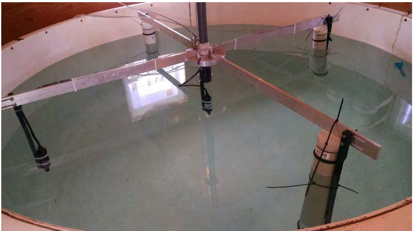
Figure 2. Experimental setup with the Ocean Sonics icTalk projector in the center of the tank, 3 C-PODs around the periphery and an Ocean Sonics icListen reference hydrophone, also at the periphery.
