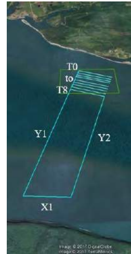
Figure 2: Historic mobile survey design. Collectively, the blue lines show one grid, with transect names indicated by the text. The green square represents the CLA.
