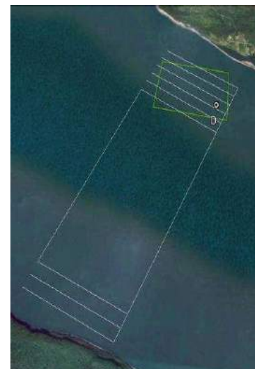
Fig. 1 Mobile survey design. The green square represents the CLA. White lines show one complete grid, with transects at the CLA (6 transects) and reference (3 transects) sites connected by cross-channel transects. The turbine is located at berth D.
