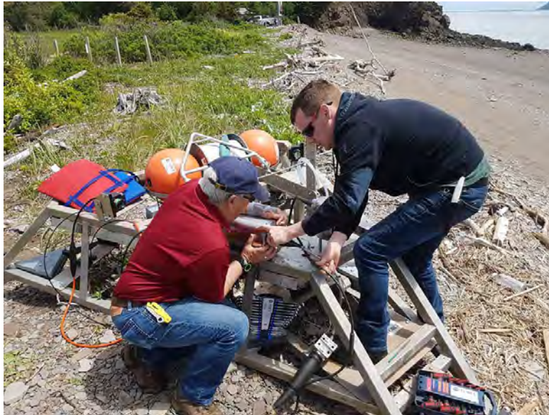
Figure 10: FORCE personnel work on the FAST-2 sensor platform in mid-June, connecting a multibeam imaging sonar camera to a multiplexer, which collects and transmits data to shore via optical fibres.
