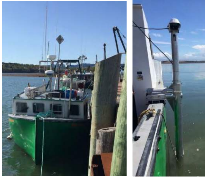
Figure 2: The Nova Endeavor at Parrsboro harbor (left) and the mounted echosounder and GPS on the side of the boat (right).
