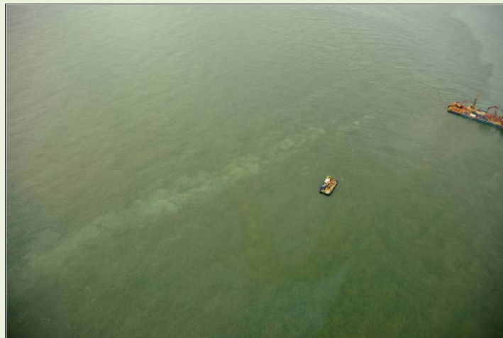
Figure 3.4: Example image of chalk sediment plumes arising from plough share dredging at the Thanet Offshore Wind Farm export cable route
