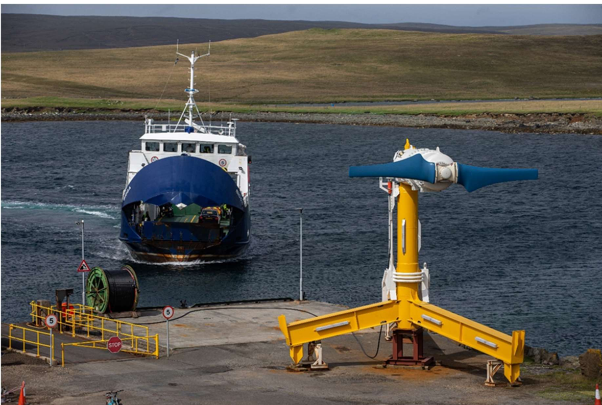
Figure 1-5 Photo of Nova Innovation’s M100-D turbine quayside before deployment in Bluemull Sound, Shetland
