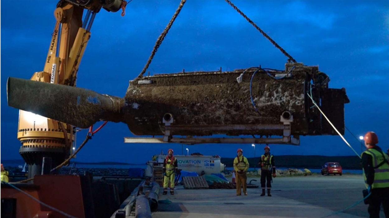
Figure 1-6 Photo of the tidal energy device after being deployed for 14 months
