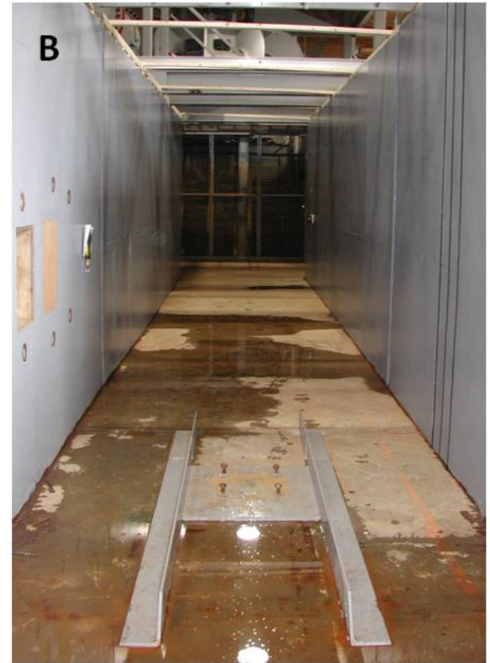
Figure 2-4 View downstream (A) and upstream (B) of the narrowed flume channel used for fish testing with hydrokinetic turbines.
