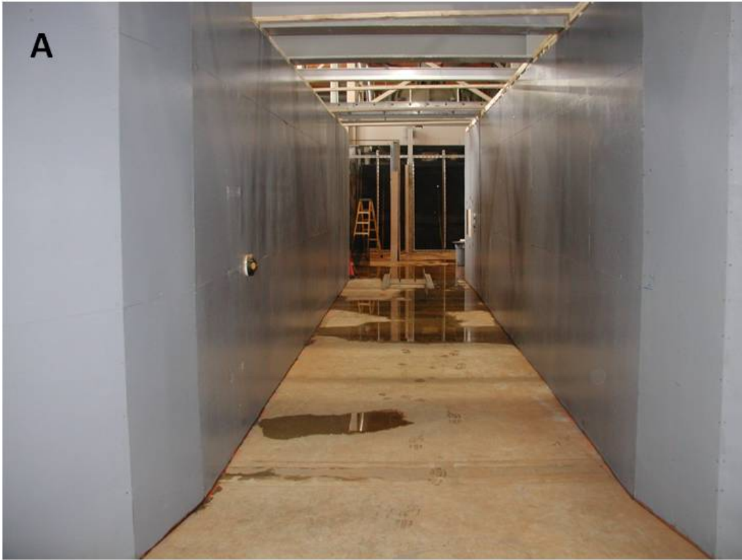
Figure 2-4 View downstream (A) and upstream (B) of the narrowed flume channel used for fish testing with hydrokinetic turbines.
