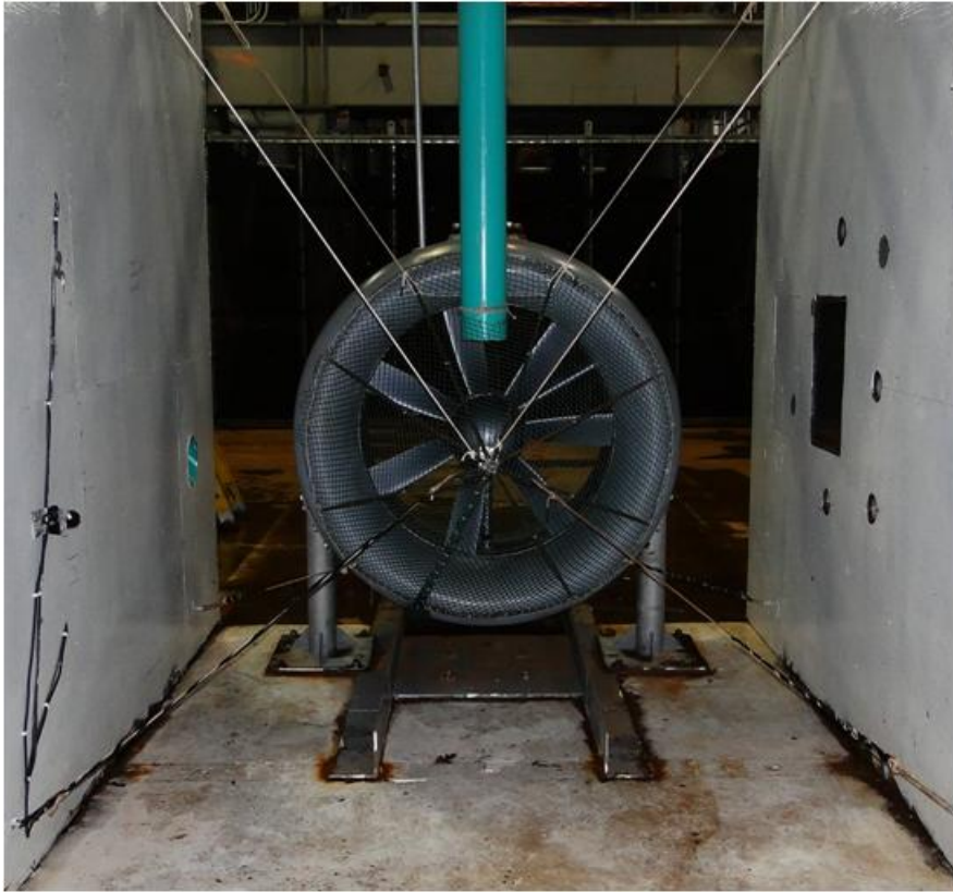
Figure 2-1 FFP's ducted axial-flow turbine installed in Alden's large flume test facility for the evaluation of fish survival and behavior (upstream side of turbine on left, downstream side on right)
