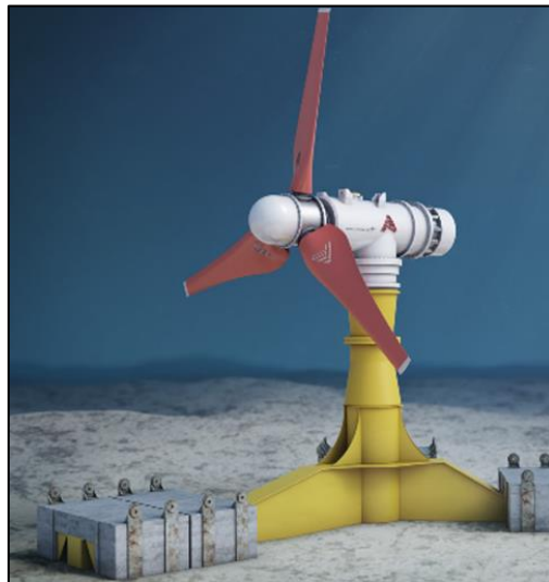
Figure 2.2. Model representation of Atlantis AR1500 horizontal axis tidal turbine installed in the Pentland Firth, Scotland.
