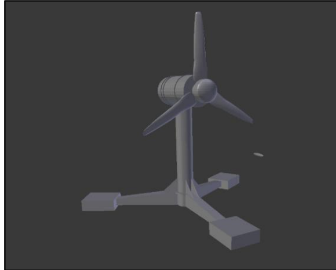
Figure 2.7. Screenshot of 3D shapefile of the horizontal axis turbine design, the ellipsoid object of the seal can be seen for scale purposes.
