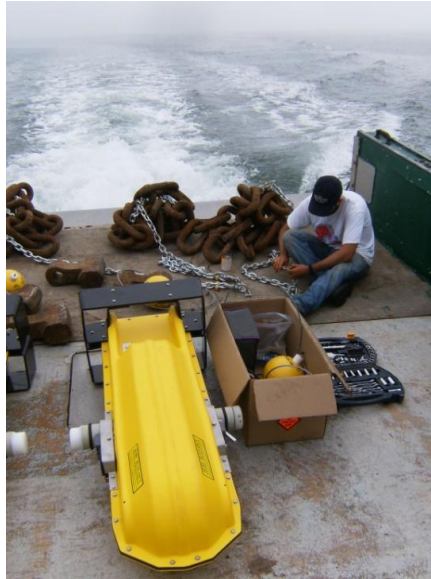
Figure 3.2. Rigging units for deployment of C-PODs. Mooring chain weights can be seen on the stern of the vessel. Photo courtesy of Colin Buhariwalla.
