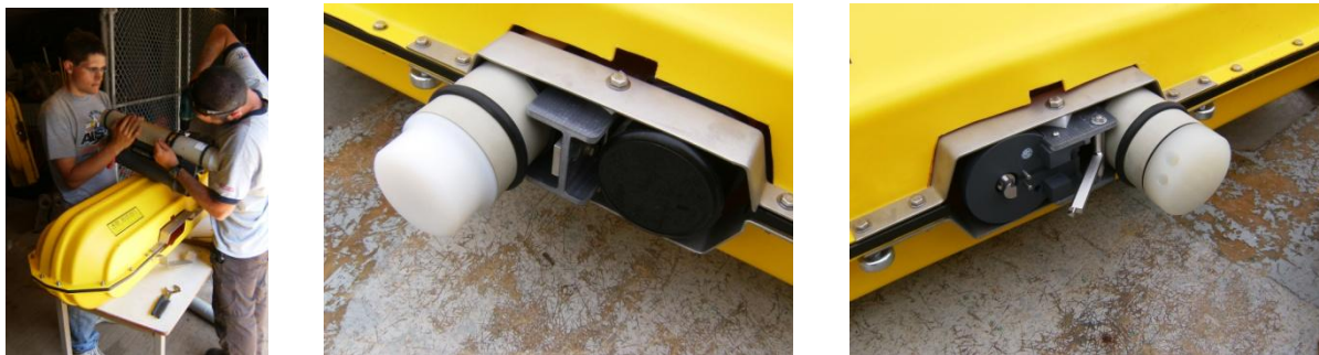
Figure 3.1. Attaching the C-POD to the acoustic release (left), and close up of the instrument package arrangement showing the top of the SUB buoy and C-POD hydrophone (centre), and the bottom of the SUB buoy showing the C-POD bottom and acoustic release point (right). Photos courtesy of Colin Buhariwalla.
