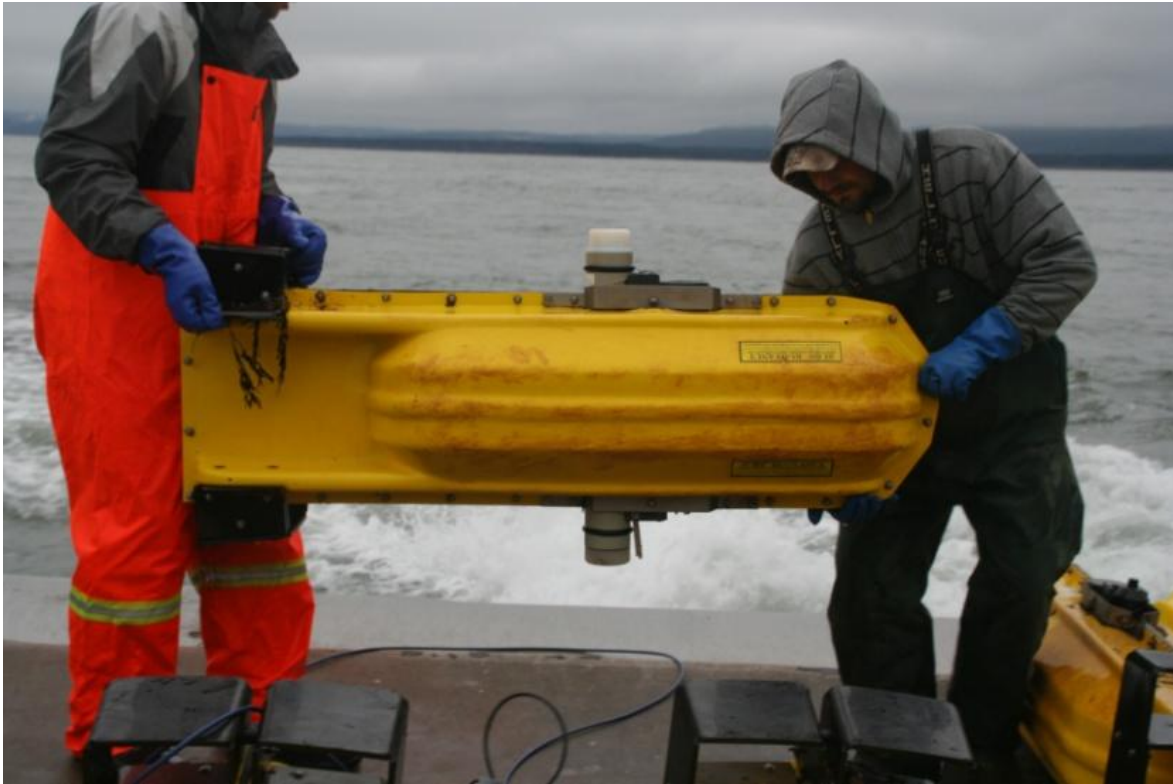
Figure 3.4. C-POD unit W1 immediately following retrieval. Note that part of the tail fin is missing. Photo courtesy of Colin Buhariwalla.
