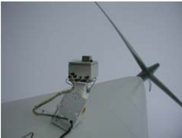
Figure 5. Thermal camera mounted with a pan/tilt head on the A2 offshore turbine at Nysted wind farm.
